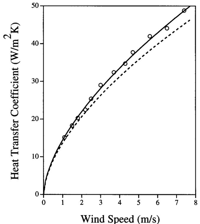
FIG. 1. The experimental values of the convective heat transfer coefficient of the face segment of the thermal simulator are plotted as a function of wind speed. The solid line is the best-fit curve, given by equation 5. The dashed line was calculated for a cylinder of the same diameter as that used by Siple and Passel for their cooling experiment in Antarctica.
