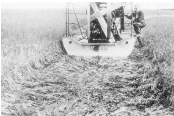
FIG. 4. Airboat and test lane used to conduct a preliminary evaluation of surface disturbance by an airboat driven back and forth 50 times over this test lane. The subsurface floating mat remained intact, although most of the emergent vegetation was removed or flattened beneath the water.
