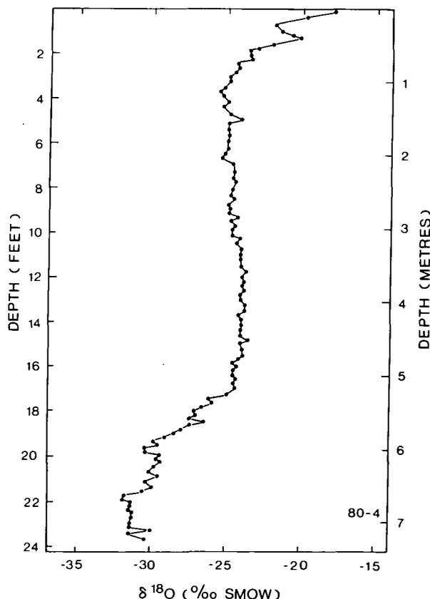
FIGURE 4. <sup>18</sup>O profile for core 80-4. Note the massive wedge of ice from 0.45 to 5.5 m.
