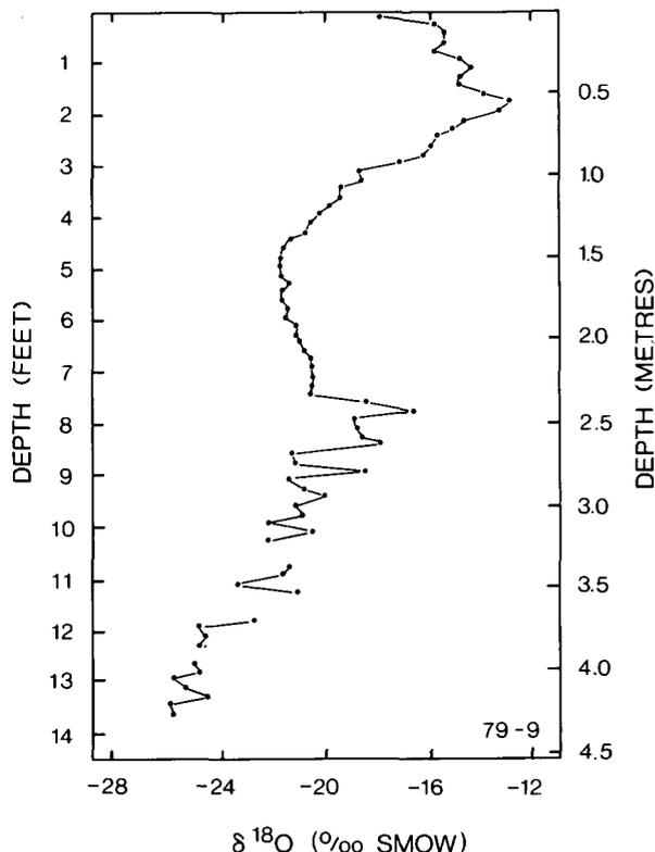
FIGURE 10.  $^{18}\text{O}$  profile for core 79-9 drilled on the control sill.
