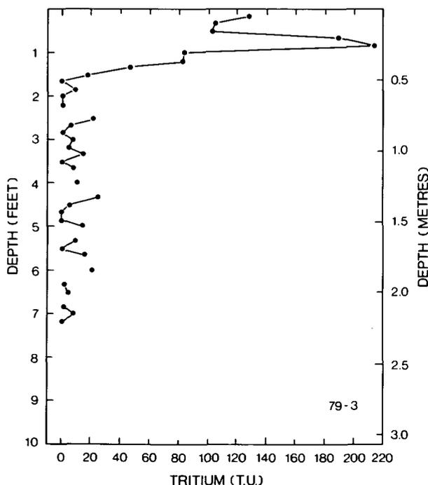
FIGURE 11. Tritium profile for core 79-3 drilled on slope outside the lake bed.
