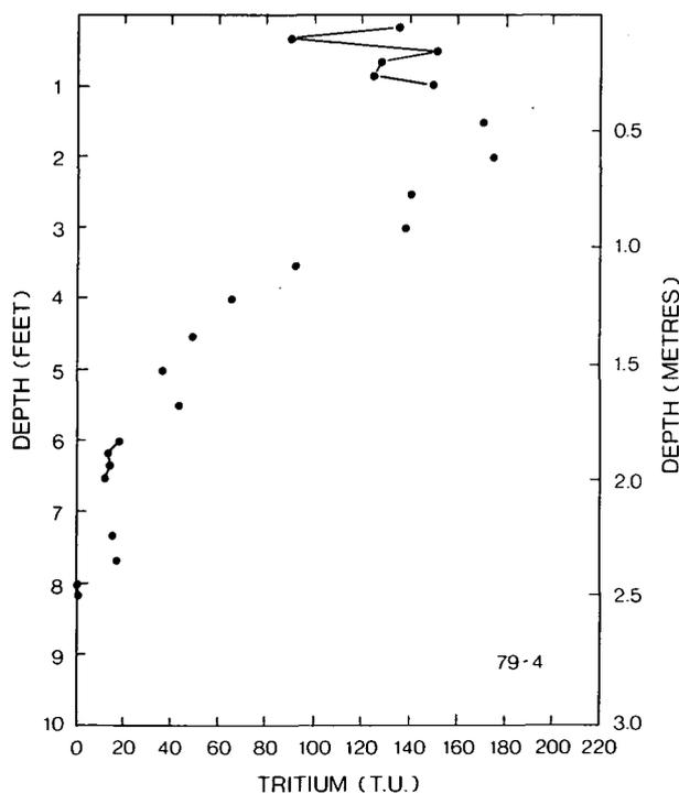
FIGURE 12. Tritium profile for core 79-4 drilled within the lake bed.
