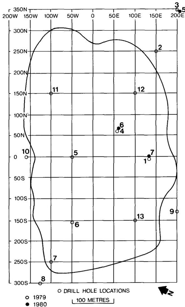
FIGURE 2. Location map of boreholes drilled at Illisarvik in 1979 and 1980.
