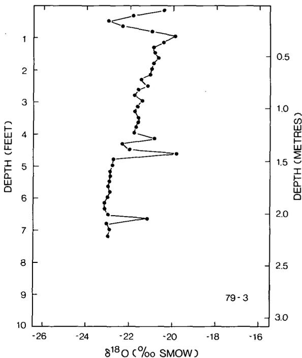
FIGURE 5.  $^{18}\text{O}$  profile for core 79-3 drilled on slope outside the lake bed.
