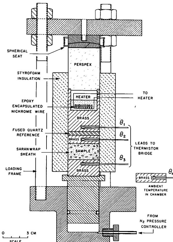
FIGURE 3. Cross-section of divided-bar thermal conductivity apparatus.
