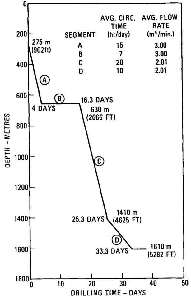
FIGURE 4. WELLTEMP drilling simulation.
