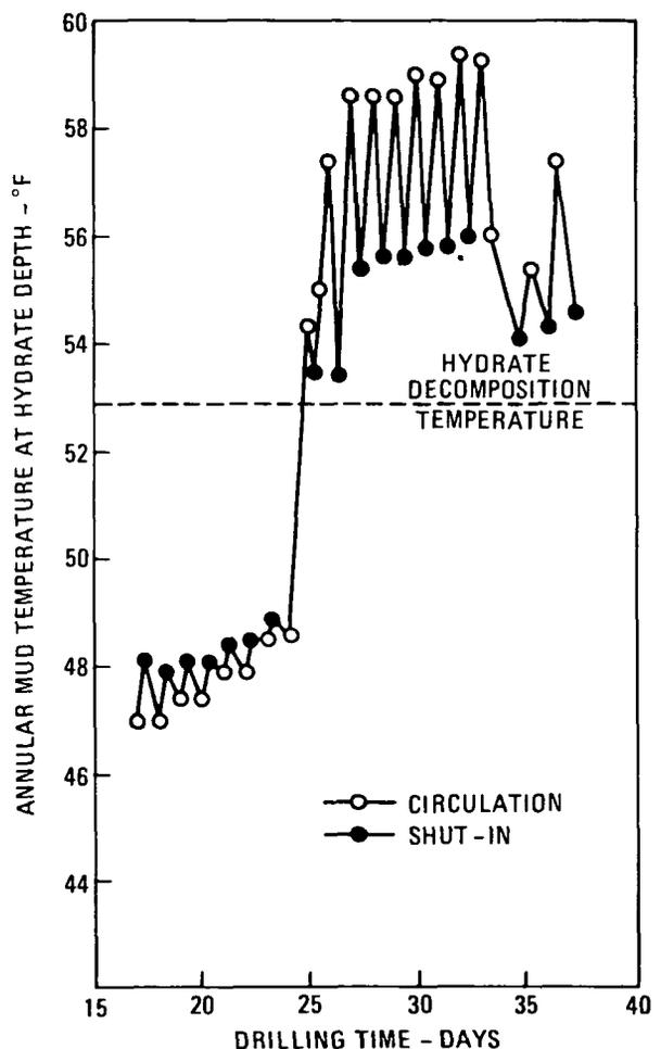
FIGURE 5. Mud temperature opposite hydrate zone.
