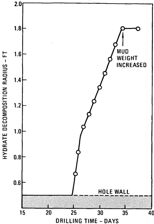
FIGURE 8. Hydrate decomposition with time.
