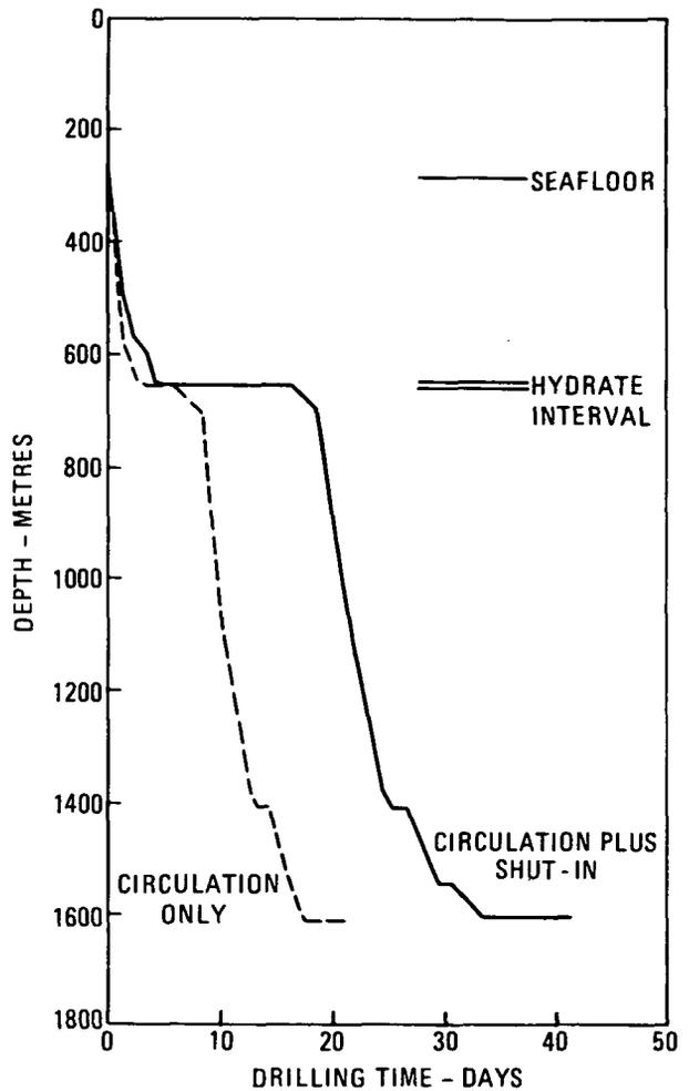
FIGURE 2. Drilling schedule for Panarctic well.
