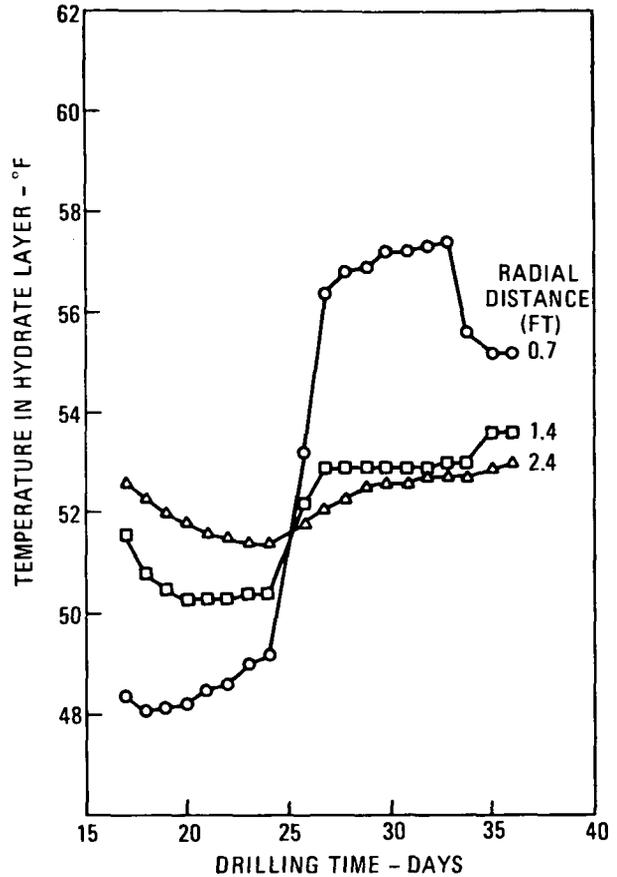
FIGURE 7. Temperature build-up in hydrate layer at various radial locations.
