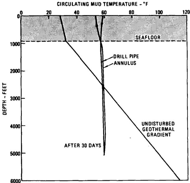
FIGURE 6. Mud temperature profile in drill pipe and annulus.
