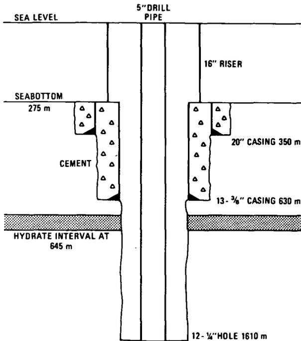
FIGURE 1. Casing program for Panarctic well.
