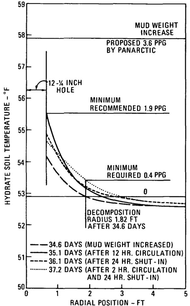
FIGURE 9. Mud weight increase for hydrate stabilization.
