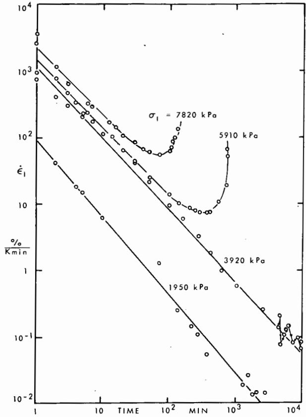
FIGURE 7. Strain rate curves for plane strain creep tests.
