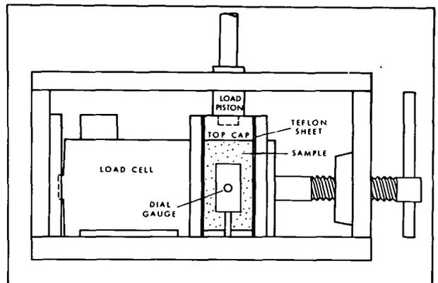
FIGURE 1. Plane strain test equipment for frozen soil.
