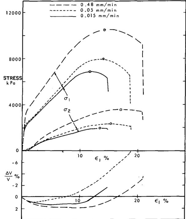
FIGURE 3. Typical stress-strain curves from rate-controlled plane strain tests.
