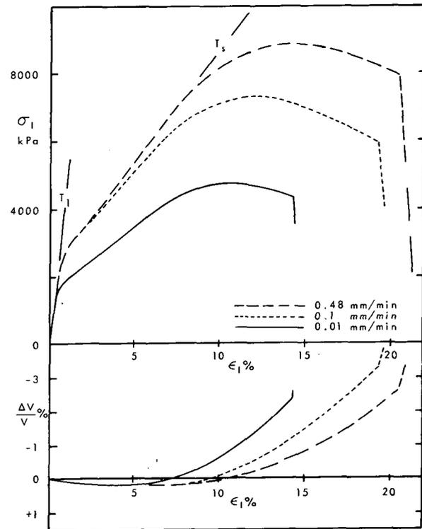
FIGURE 2. Typical stress-strain curves from rate-controlled unconfined triaxial tests.
