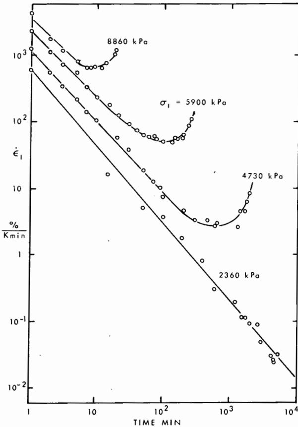
FIGURE 6. Strain rate curves for triaxial creep tests.
