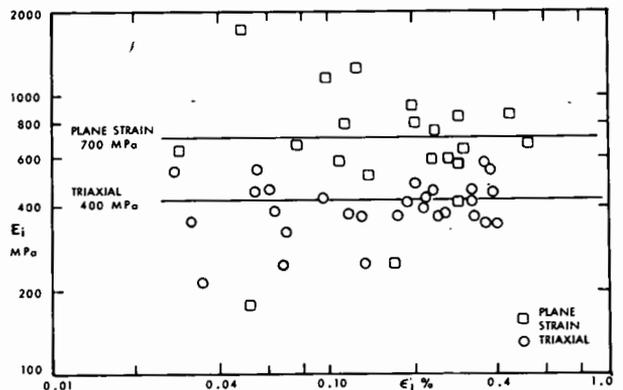
FIGURE 8. Tangent moduli from displacement-controlled tests.
