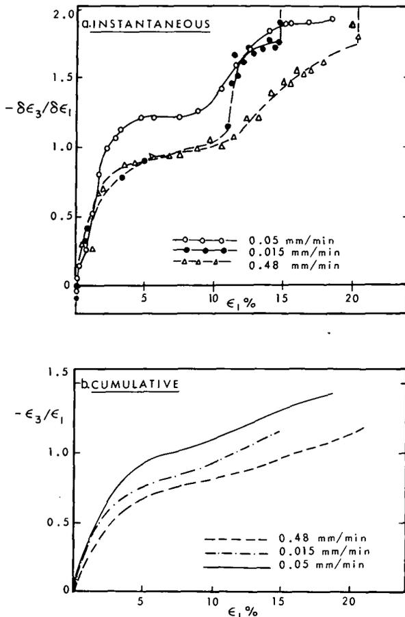
FIGURE 4. Strain ratios during plane strain tests.
