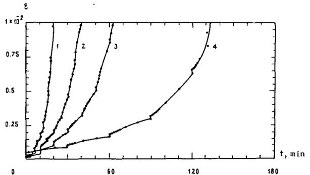
FIGURE 4. Relationship  $\epsilon$  vs.  $t$  for step loading with a stress step value  $\Delta\sigma = 0.2$  MPa and durations of loading  $t$  of 2 (1), 5 (2), 10 (3), and 30 (4) min.
