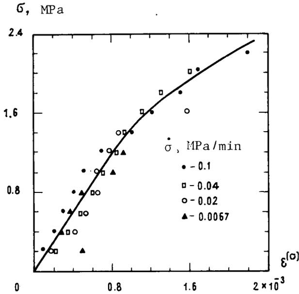
FIGURE 5. Relationship  $\sigma$  vs.  $\epsilon^{(c)}$  for step loading.
