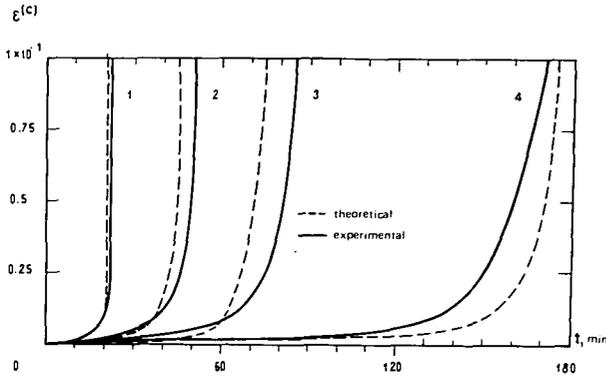
FIGURE 11. Theoretical and experimental relationships  $\epsilon^{(c)}$  vs.  $t$  for step loading at the following rates of loading  $\dot{\sigma}$  in MPa/min: 0.1 (1); 0.04 (2); 0.02 (3); and 0.0067 (4).
