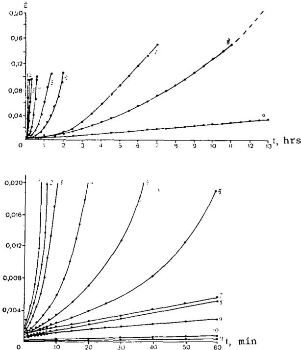
FIGURE 1. Creep curves of ice at stresses  $\sigma$ , in MPa, equal to the following: 2.295 (1); 2.04 (2); 1.53 (3); 1.275 (4); 1.02 (5); 0.89 (6); 0.765 (7); 0.64 (8); 0.51 (9); 0.25 (10); and 0.15 (11).
