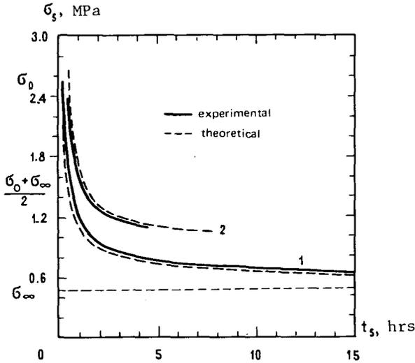
FIGURE 13. Theoretical and experimental curves for the long-term failure of ice under the following test conditions:
