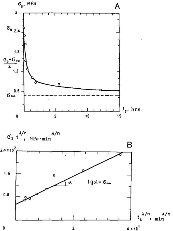
FIGURE 2. a Curve for long-term failure of ice. b Determination of parameters  $\sigma_\infty$  and  $A^{1/n}$ .
