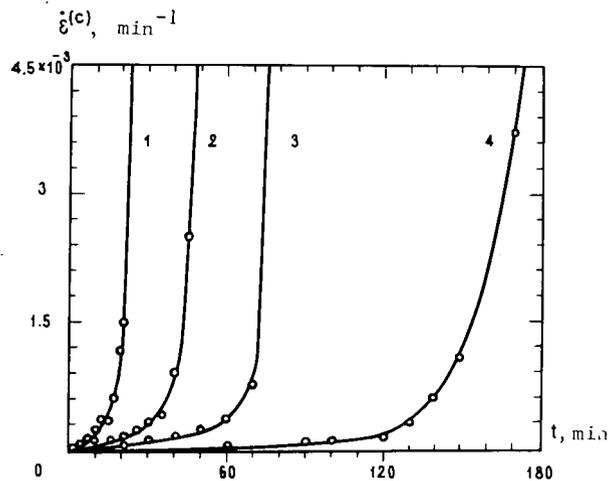
FIGURE 6. Relationships  $\dot{\epsilon}^{(c)}$  vs.  $t$  for step loading at the following rates of loading  $\dot{\sigma}$  in MPa/min: 0.1 (1); 0.04 (2); 0.02 (3); 0.0067 (4).
