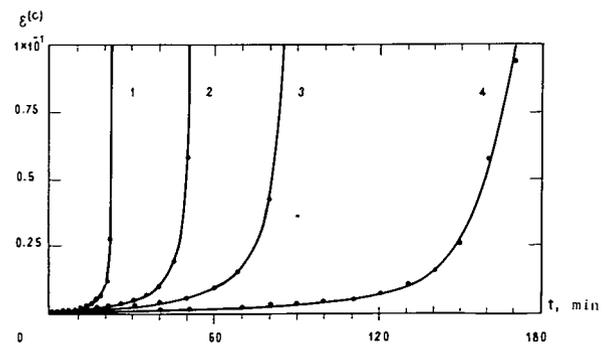
FIGURE 7. Relationships  $\epsilon^{(c)}$  vs.  $t$  for step loading at the following rates of loading  $\dot{\sigma}$  in MPa/min: 0.1 (1); 0.04 (2); 0.02 (3); 0.0067 (4).
