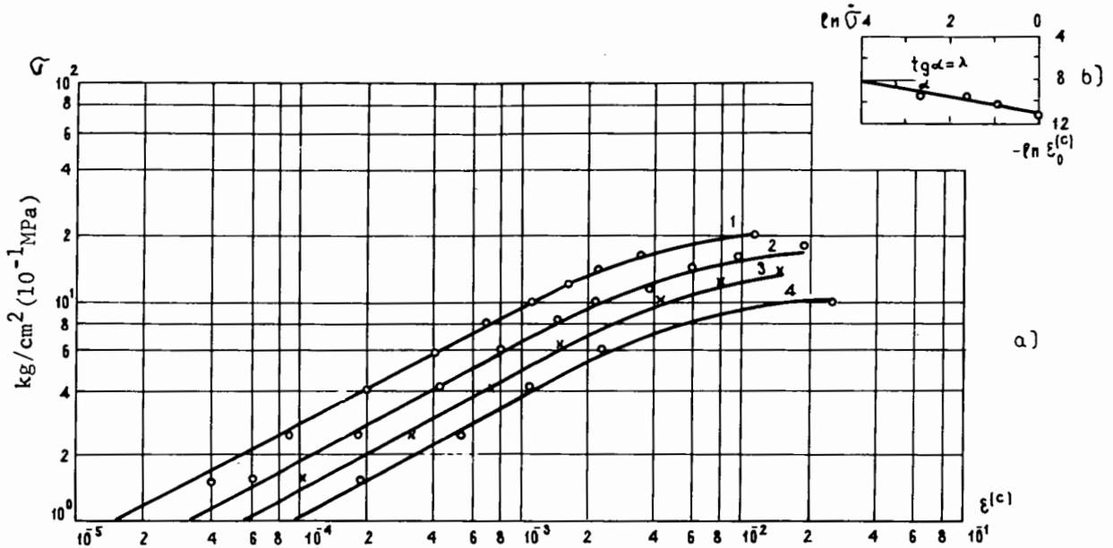
FIGURE 8. Relationships  $\sigma$  vs.  $\epsilon^{(c)}$  for step loading in logarithmic co-ordinates at the following rates of loading  $\dot{\sigma}$  in MPa/min: 0.1 (1); 0.04 (2); 0.02 (3); 0.0067 (4).
