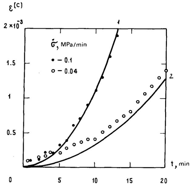
FIGURE 12. Theoretical and experimental relationships  $\epsilon^{(c)}$  vs.  $t$  for the rates of loading  $\dot{\sigma}$  in MPa/min of 0.1 (1) and 0.04 (2) (initial segments of curves).
