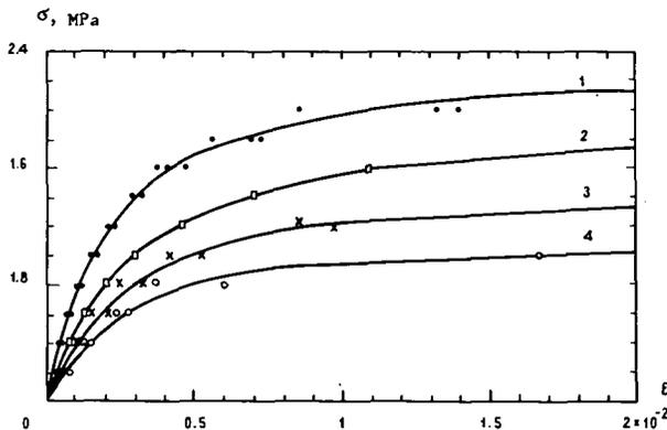
FIGURE 3. Relationship  $\sigma$  vs.  $\epsilon$  for step loading with a stress step value of  $\Delta\sigma = 0.2$  MPa for a duration of loading  $t$ , equal to 2 (1), 5 (2), 10 (3), and 30 (4) min.
