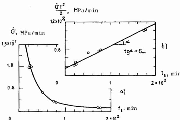
FIGURE 9. a) Loading rate  $\dot{\sigma}$  vs. time to failure  $t_f$ ; and b) determination of parameters  $\sigma_{\infty}$  and  $A$ .
