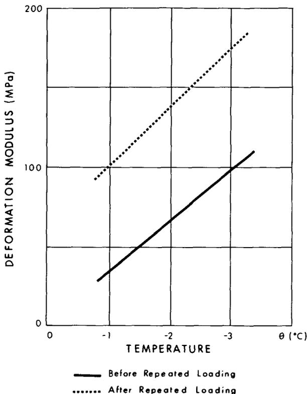
FIGURE 3. Influence of repeated loading on the deformation modulus at various temperatures.
