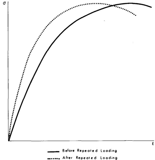
FIGURE 1. Influence of repeated loading on the stress-strain curve.
