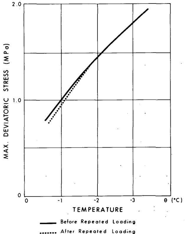
FIGURE 2. Influence of repeated loading on the shear strength at various temperatures.
