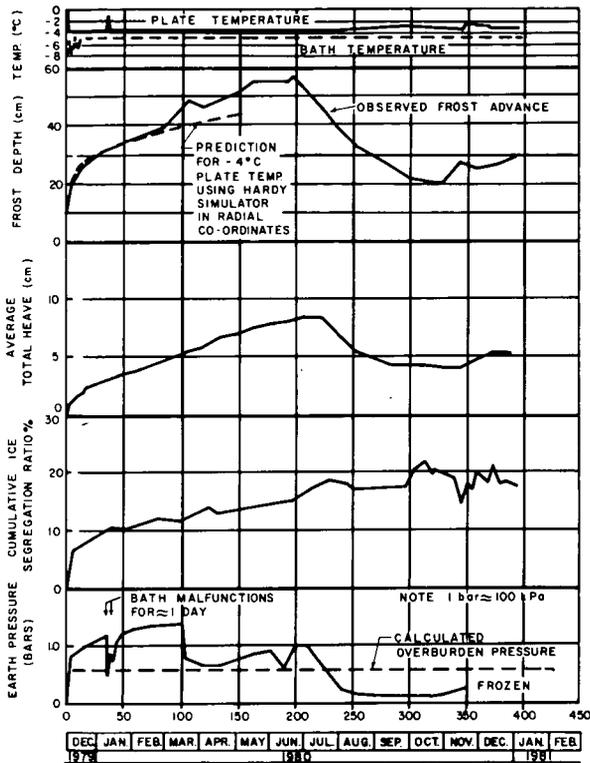
FIGURE 7. Frost heave test data for Calgary Plate 7.
