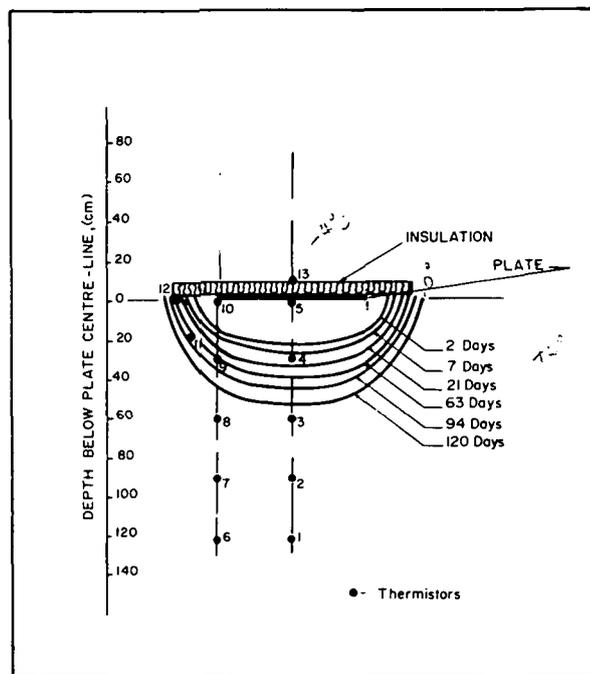
FIGURE 6. Advance of frost bulb at Calgary Plate 7.
