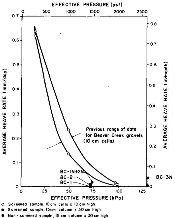
FIGURE 11. Beaver Creek gravel heave rate versus effective stress small- and large-diameter lab test data.
