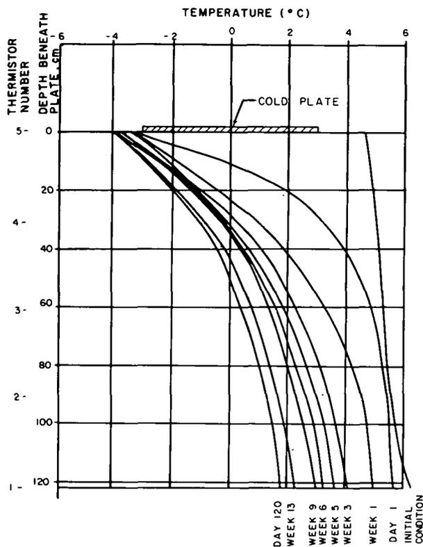
FIGURE 5. Temperature profile beneath centre-line of Calgary Plate 7.
