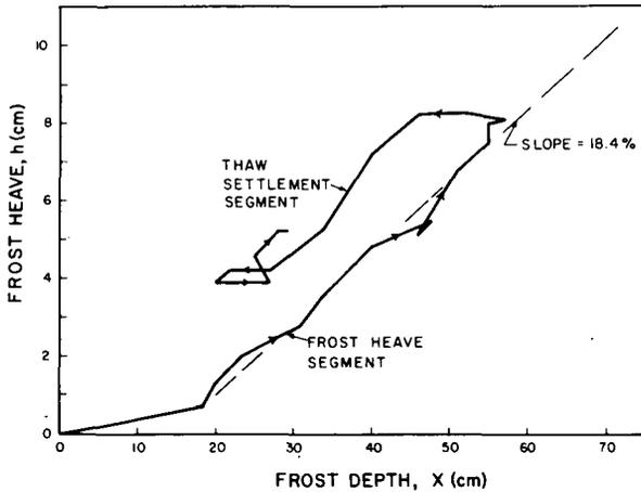
FIGURE 10. Heave-frost depth plot for Calgary Plate 7.
