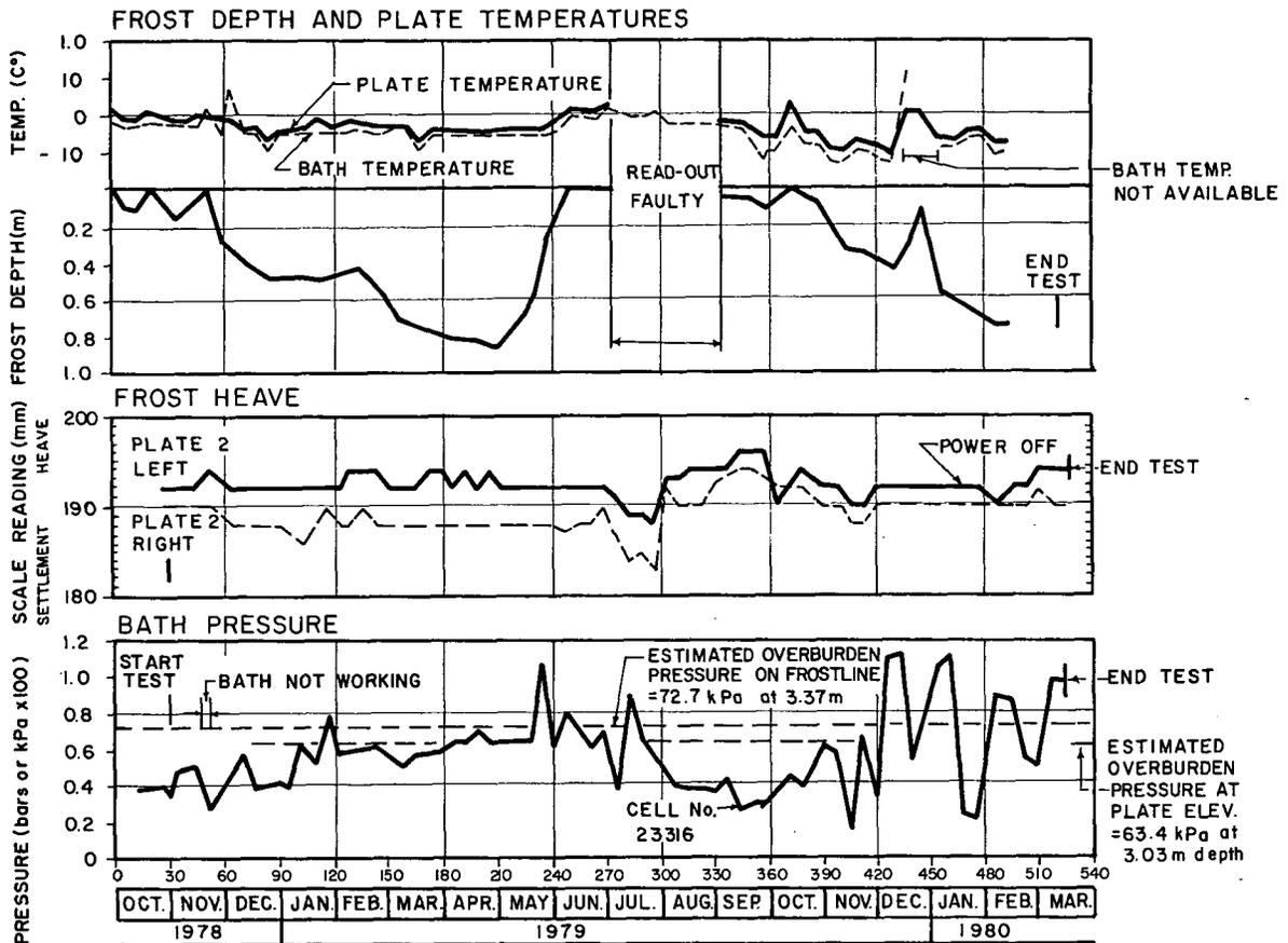
FIGURE 9. Frost heave test data for Beaver Creek Plate 2.
