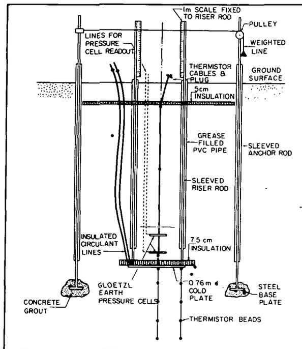
FIGURE 3. Cold plate installation.
