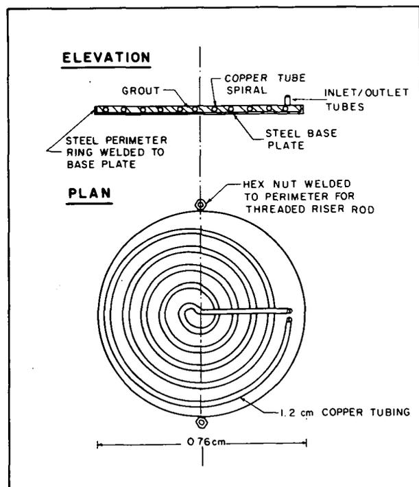
FIGURE 2. Cold plate fabrication.
