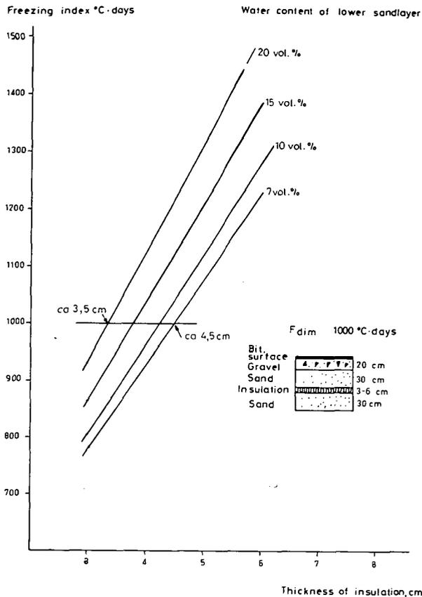
FIGURE 3. The frost resistance capacity of a road base with polystyrene foam for different values of the water content of the material in the layers just beneath the foam layer, expressed as a function of the thickness of the foam layer.
