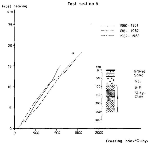
FIGURE 5. Frost heaving in relation to freezing index for the Test Road Öjebyn 1957 in the north of Sweden.
