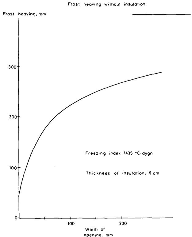
FIGURE 6. Frost heaving as a function of the width of parallel openings between plastic foam boards. The width of the boards is 60 cm and their thickness 6 cm, and the freezing index is 1435 °C · days.
