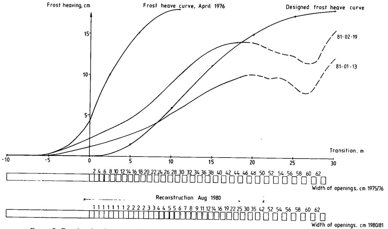
FIGURE 7. Frost heaving along a transition with successive widening of the openings between the plastic foam boards.
