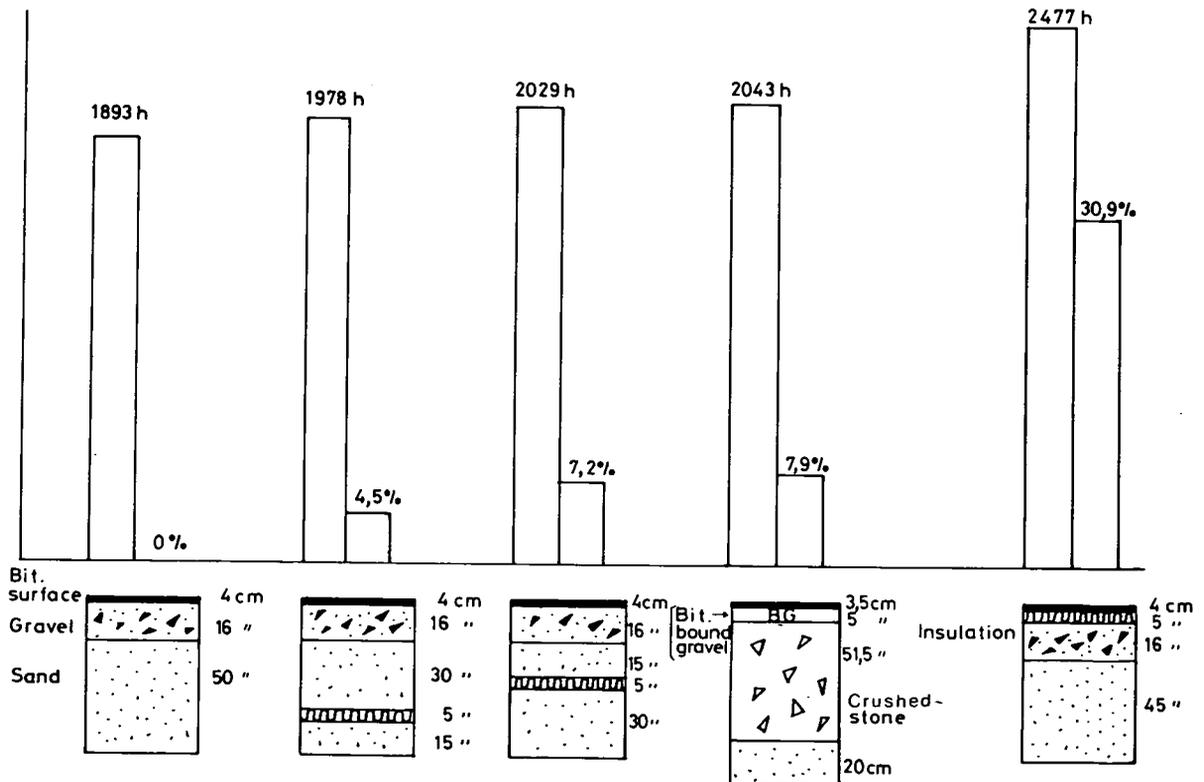
FIGURE 8. Duration of time with surface temperature below  $-2^{\circ}\text{C}$  for some road bases, indicating different degree of risk for surface icing (from Gustavsson 1981).
