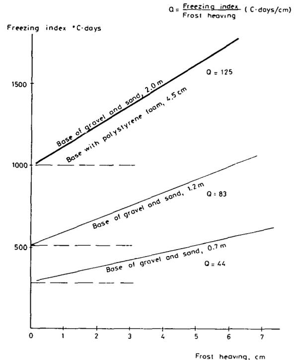
FIGURE 4. Calculated frost heaving in relation to freezing index (after S. Fredén: *Pers. Commun.* 1980).
