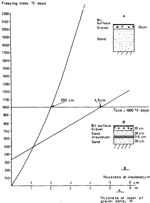
FIGURE 1. The calculated frost resistance capacity of a sand-gravel road base and a base frost protected with polystyrene foam. These capacity values are not to be generally used. By calculating the frost resistance capacity for any single base the appropriate input values have to be chosen.
