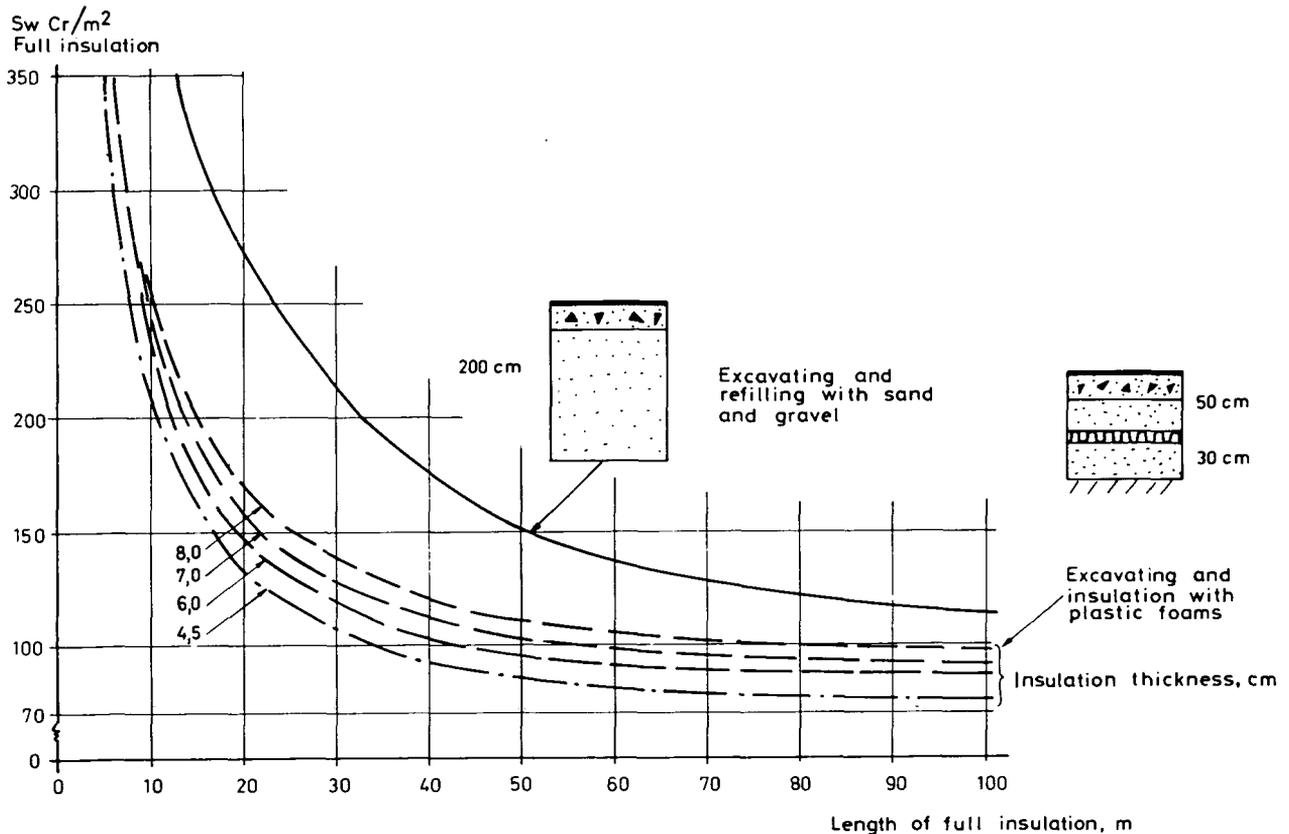
FIGURE 9. Calculated construction costs for repairing roads in the north of Sweden when excavating the poor material *in situ* and refilling it by pure sand-gravel material and polystyrene foam.
