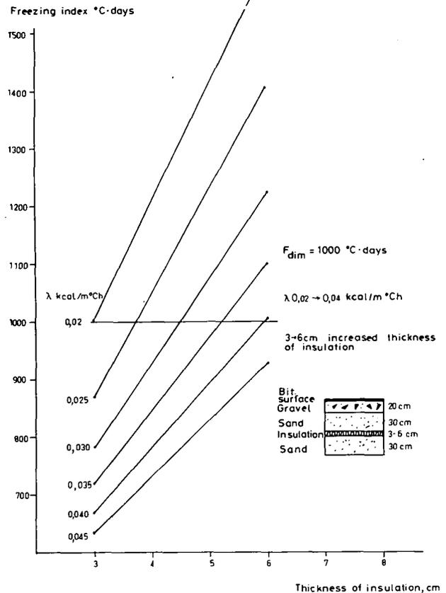
FIGURE 2. The frost resistance capacity of a road base with polystyrene foam expressed, for different values of the thermal conductivity, as a function of the thickness of the foam layer.
