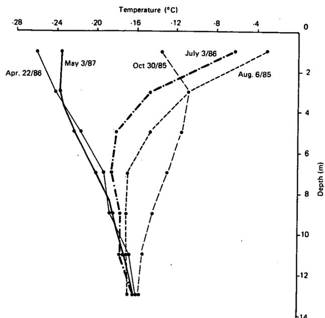
Figure 2. Ground temperature conditions at Rea Point between August 1985 and May 1987.
