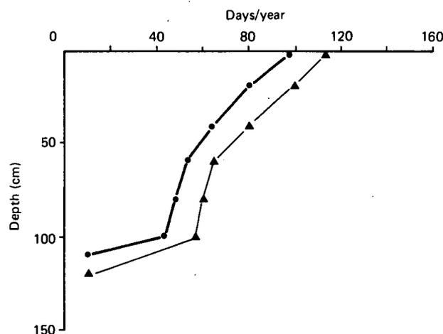
Figure 3. Maximum and minimum numbers of days with soil temperatures greater than  $-3.0^{\circ}\text{C}$  (all study sites).
