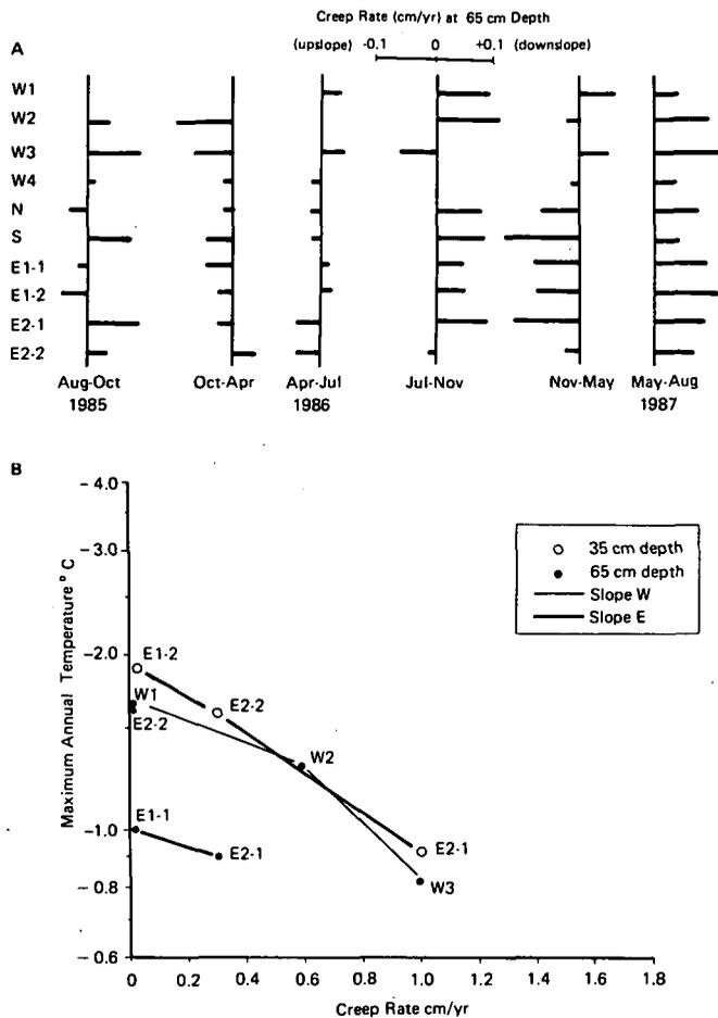
Figure 5. Variability of creep rates: A) Diagram showing discrete time periods and creep rates at 65 cm depth for six discrete time periods; B) Diagram showing creep rates at 35 and 65 cm depth in relation to maximum annual ground temperatures (log scale) on east and west-facing slopes. Straight lines represent possible exponential relationships between creep rate and temperature.
