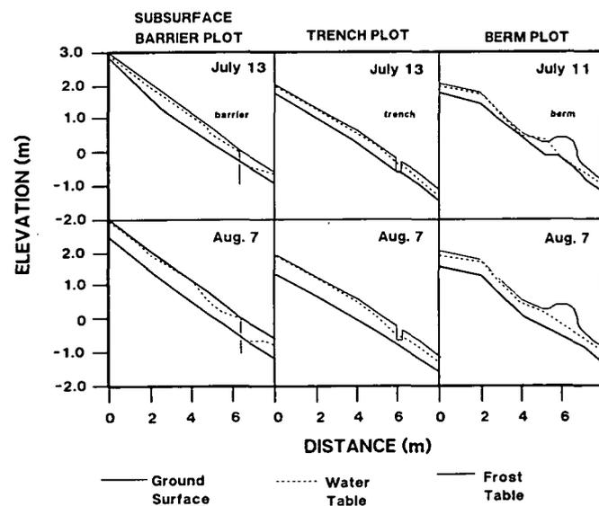
Figure 5. Profiles of the slope, water table and frost table at the treatment sites in mid-July and early August, 1988.
