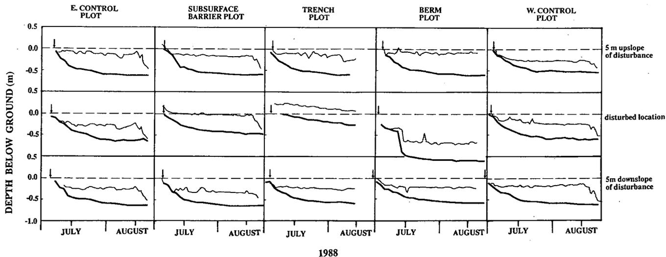
Figure 4. Fluctuations of water table (dotted lines) and frost table (full lines) at the experimental plots between July 1 and August 23, 1988. Surface runoff occurred when the water table was above the ground, except in the trench where water was ponded. Arrows indicate dates when particular sites became snow-free.
