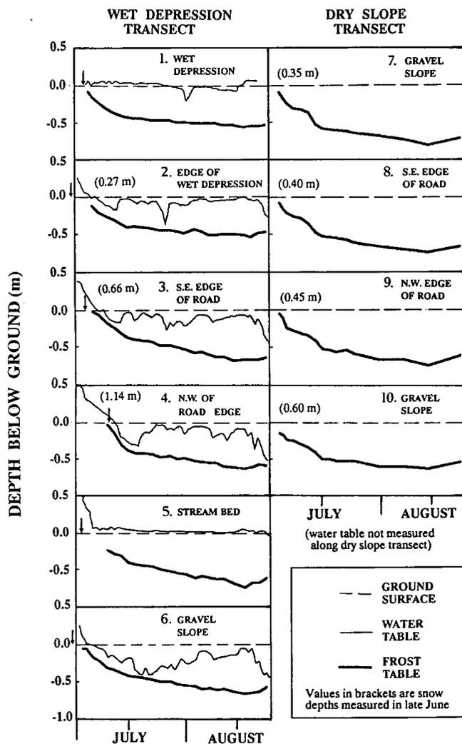
Figure 6. Fluctuations of water table and frost table along transects across the gravel road. Numbers refer to the locations shown in Figure 2, and arrows indicate dates when particular sites became snow-free.
