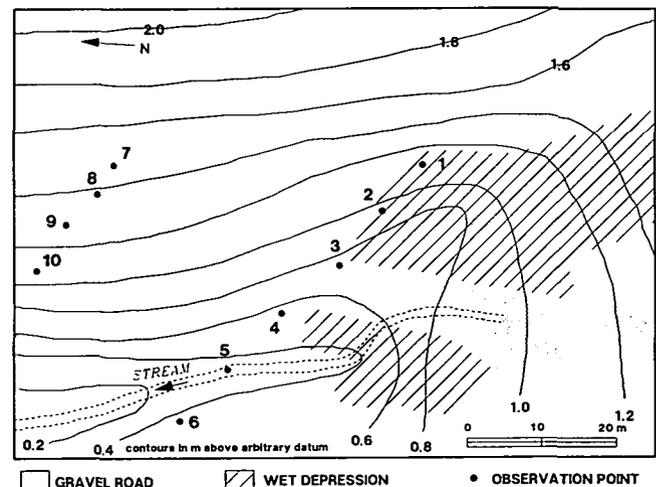
Figure 2. Gravel road crossing at wet depression site. Numbers refer to various groundwater wells.
