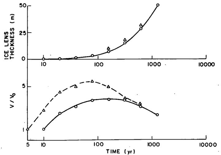
Fig. 4 Prediction of ice lens growth in coarse-grained soils
