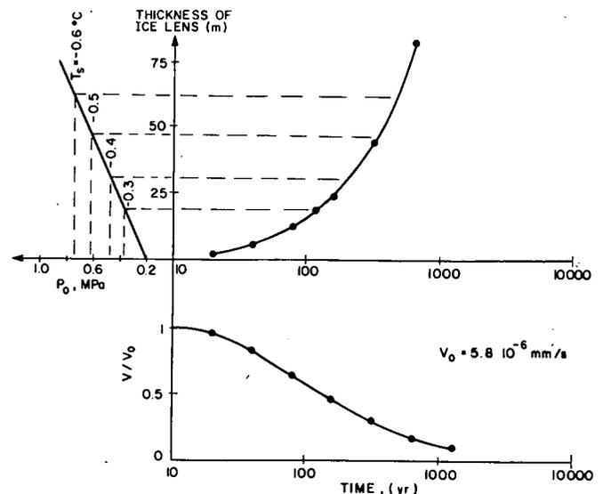
Fig. 3. Prediction of ice lens growth in frost susceptible soils. The following values were used in the simulation:  $\alpha = 10^{-4}$  cm<sup>2</sup>/s;  $T_c = -20$  °C;  $T_o = 2$  °C;  $K_u = 1.46$  mW/mm °C;  $K_f = 1.76$  mW/mm °C;  $K_i = 2.2$  mW/mm °C;  $t_o = 10$  years
