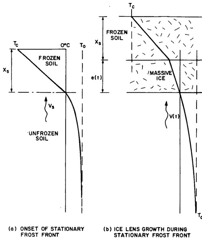
Fig. 2. Schematic of the temperature distribution in the semi-infinite domain
