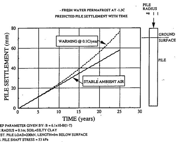
**Figure 6. Predicted pile settlement for fresh water permafrost.**
