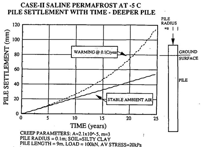
Figure 10. Pile settlement in saline permafrost-deeper pile.
