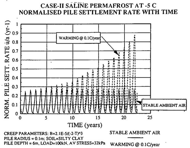
**Figure 8. Pile creep rates for saline permafrost.**
