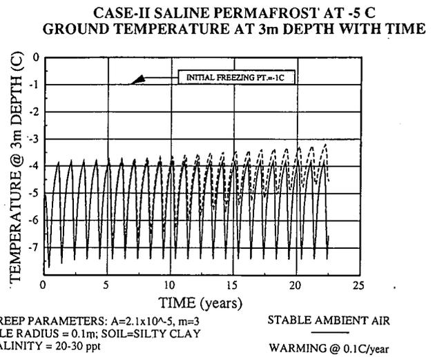
**Figure 7. Predicted ground temperatures in saline permafrost.**
