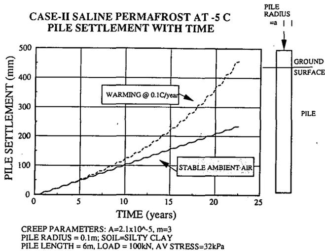
Figure 9. Predicted pile settlement for saline permafrost.
