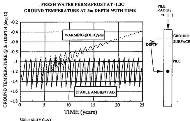
Figure 4. Effect of climatic warming on predicted ground temperatures.
