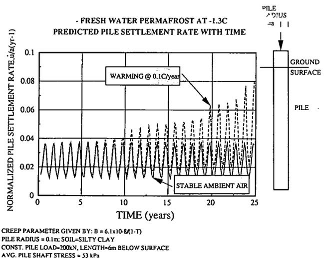
Figure 5. Pile creep rates for fresh water permafrost.
