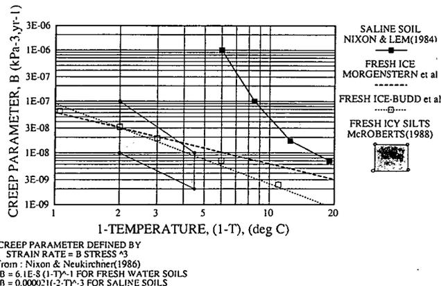
Figure 3. Creep parameter,  $B$ , for frozen soils correlated with temperature.
