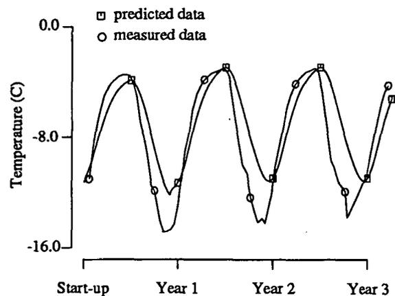
Figure 5. Measured and predicted temperatures between water and sewer pipes at station 1+60 along Stevenson Street.
