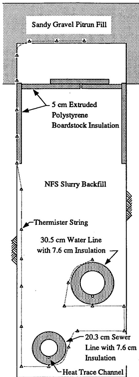
Figure 1. Typical trench configuration for water and sewer lines in a common trench, Phase I, direct-bury utilities system.
