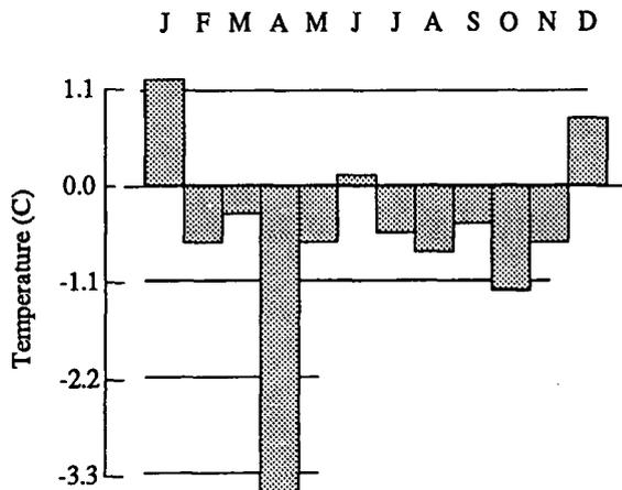
Figure 2. Long-term average monthly air temperatures used for computer modeling minus average monthly air temperatures measured during direct-bury system operation.
