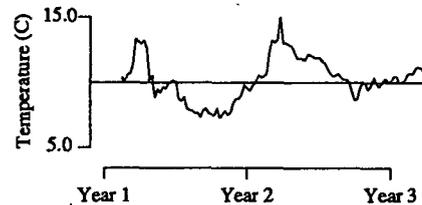
Figure 4. Measured water temperatures after cooling in shortest loop of direct-bury system. Note that data for first year are not available.
