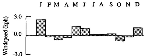
Figure 3. Long-term average monthly windspeeds used for computer modeling minus average monthly windspeeds measured during direct-bury system operation.
