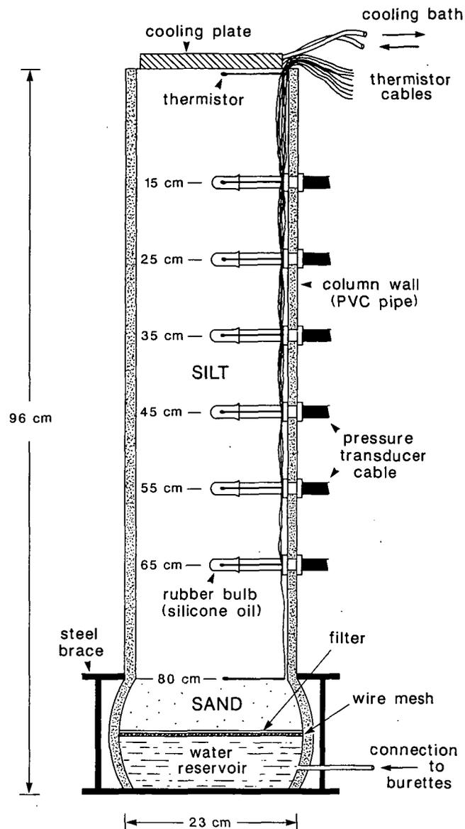
Figure 2. Schematic diagram of soil column experiment.
