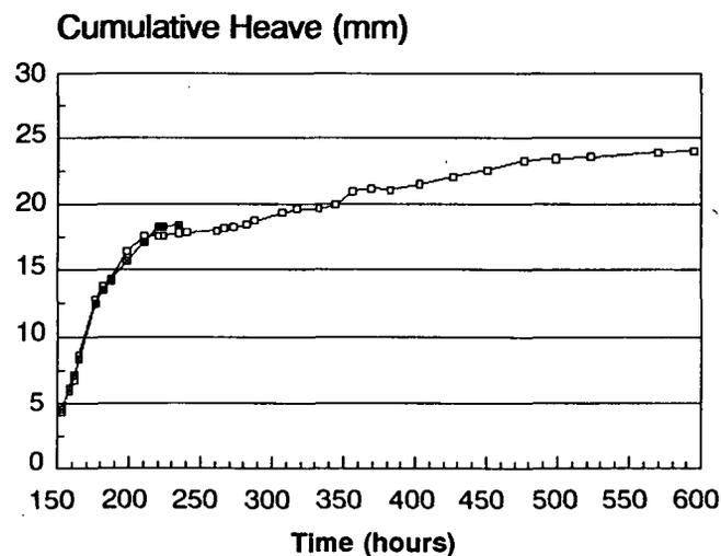
Figure 5. Cumulative heave, soil column experiment (note that heave values after 250 hours are based on calculation using water inflow measurements, since the dial gauge malfunctioned after that time; both sets of data are shown up to 250 hours.).
