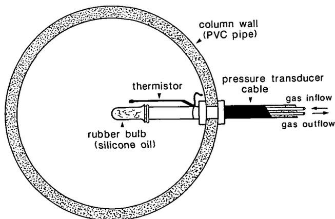
Figure 1. Top view of soil column assembly.
