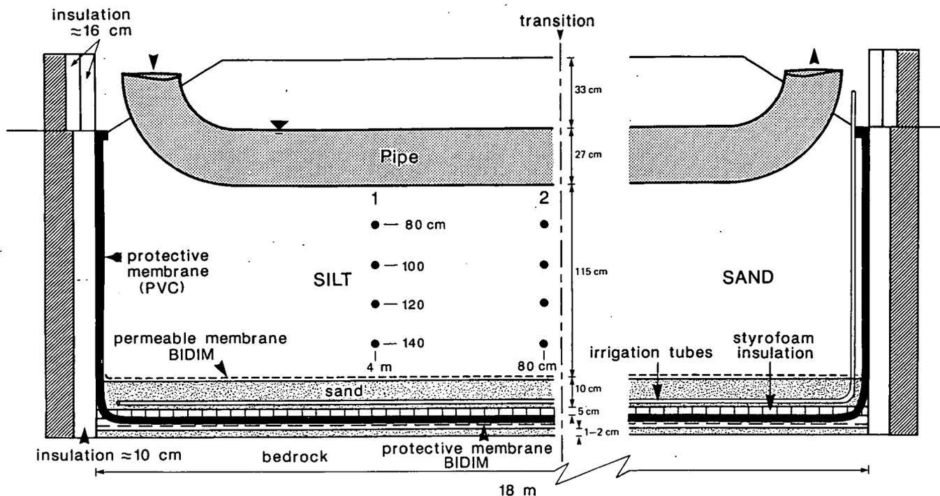
Figure 3. Longitudinal cross-section of the Caen experiment.
