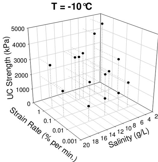
Figure 6. 3D Scatter graph for T= -10°C
