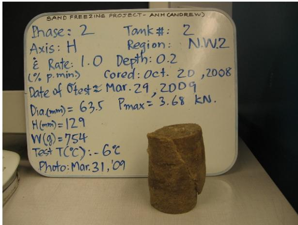
Figure 5. A sample after the strength test
