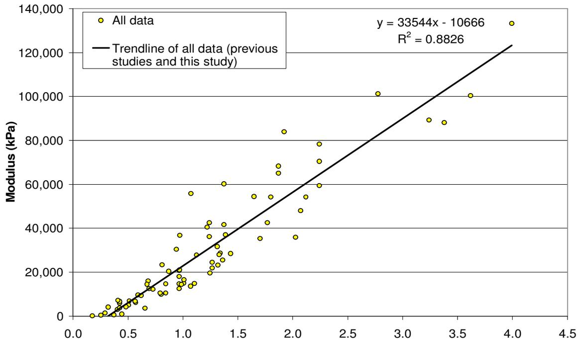
Figure 12. Correlation of modulus  $E_s$  versus  $[S^{-a} \times \dot{\epsilon}^b \times (-T)^c]$  presented with all sets of data
