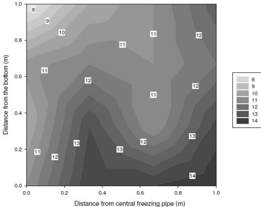
Figure 13. Final salinity distribution in a tank having initial salinity of 20 g/L (left side is the central freezing pipe)
