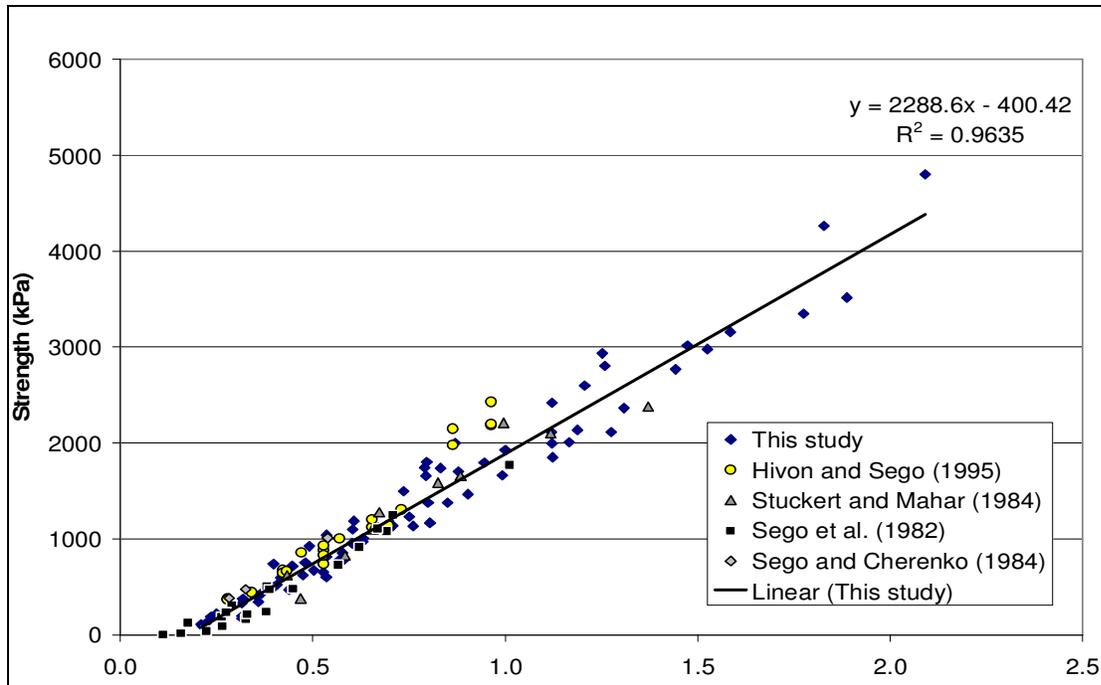
Figure 10. Correlation of compressive strength  $\sigma$  (kPa) versus  $(-T)^m \times \dot{\epsilon}^n \times \left(\frac{1}{S}\right)^p$
