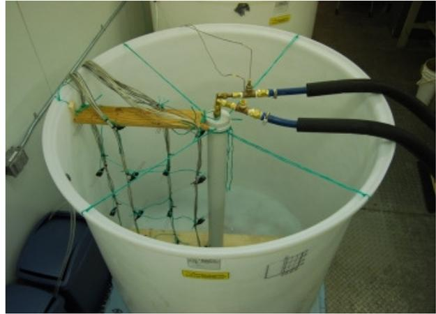
Figure 1. Instrumentation before sand filling
