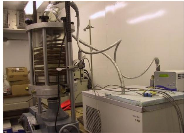
Figure 4. Modified cell used for UC strength test of FSS
