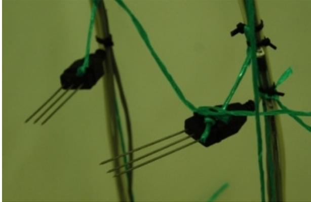
Figure 3. Thermistors and TDR probes in the tank
