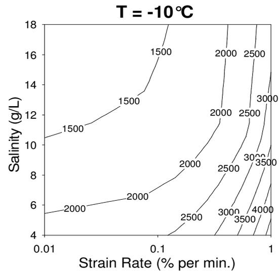
Figure 8. Contour graph for UC strength at T= -10°C
