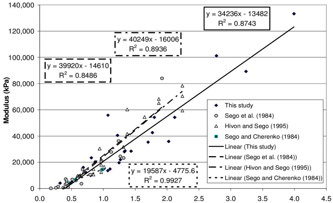
Figure 11. Correlation of modulus  $E_s$  versus  $[S^{-a} \times \dot{\epsilon}^b \times (-T)^c]$  presented in separate sets of data
