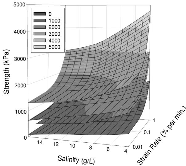
Figure 9. 3D surface plots for UC strengths at  $T = -10^{\circ}\text{C}$ ,  $-6^{\circ}\text{C}$ ,  $-4^{\circ}\text{C}$  and  $-2^{\circ}\text{C}$  from top down respectively
