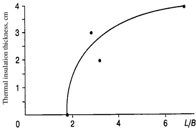
Figure 5. The dependence of on the ratio of embankment surfaces. Dots are the result of modeling.
