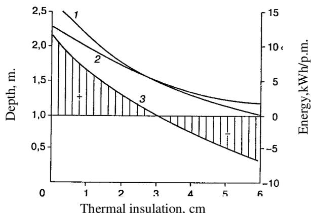
Figure 2. Dependence of the depth of thawing (1) and freezing (2) of the soil on the escarpment and the specific heat energy (3) on the insulation thickness: (PK 6711+00, H=6.0 m, L/B=3.04).
