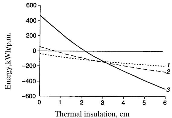
Figure 1. Dependence of the total thermal energy penetrating into the foundation of the embankment on the thickness of thermal insulation on its escarpments: 1 – PK 6710+00,  $H=3.5$  m,  $L/B = 1.94$ ; 2 – PK 6711+00,  $H=6.0$  m,  $L/B=3.04$ ; 3 – PK 6710+50,  $H=9.5$  m,  $L/B=6.72$ .
