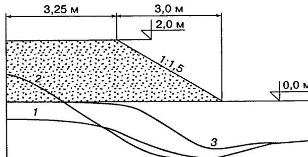
Figure 3. The position of the upper boundary of the permafrost soils in the body and foundation of the embankment at the end of summer season 50 years after its construction (PK 6692+00, H=2.0 m, L/B-1.11): 1 – embankment without thermal insulation, 2,3 – embankment with 12 cm insulation laid horizontally (2 – on the surface of the subgrade covering all its width, 3 – at the height of 0.3 m from the embankment footing covering all its width).
