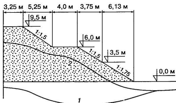
Figure 4. The position of the upper boundary of the permafrost soils in the body and foundation of the embankment at the end of summer season 50 years after its construction (PK 6710+50, H=9.5 m, B=6.5 m, L=39.7 m): 1 – embankment without thermal insulation, 2 – embankment with 4 cm thick thermo insulation laid under the paving of the escarpment throughout their length.
