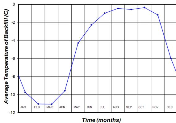
Figure 2. Average Temperature of the Soil Above the Pipe
