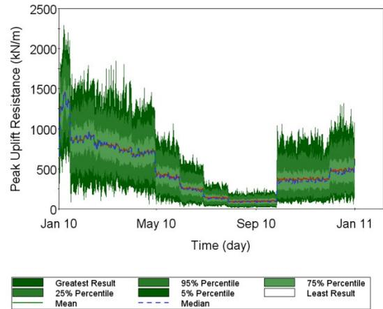
Figure 15. Variation of Peak Uplift Resistance with Time
