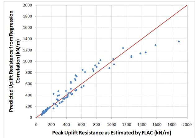
Figure 8. Peak Uplift Resistance as Predicted by Regression Correlation versus Peak Uplift Resistance as Estimated from FLAC modelling.
