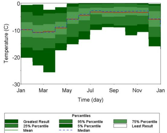
Figure 10. Variation of Soil Temperature with Time
