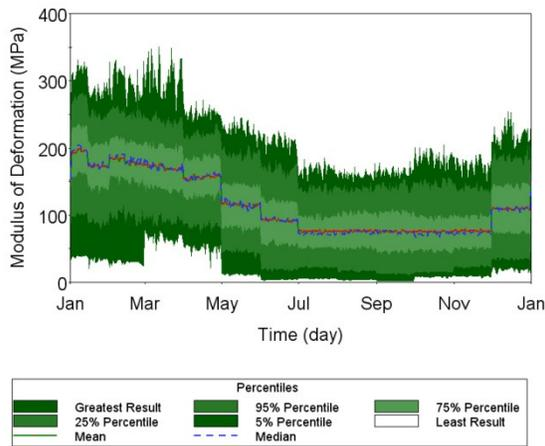
Figure 12. Variation of the Modulus of Deformation with Time
