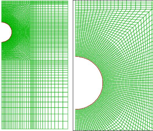
Figure 7. FLAC Model Mesh, Full View (left) and Close Up (right) (Liu et. al 2004)
