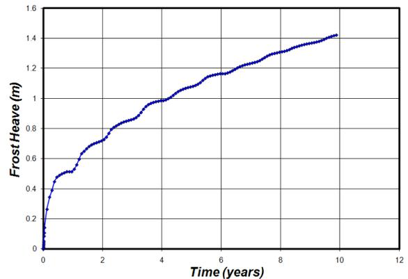
Figure 3. Frost Heave of Hypothetical Pipe with Time
