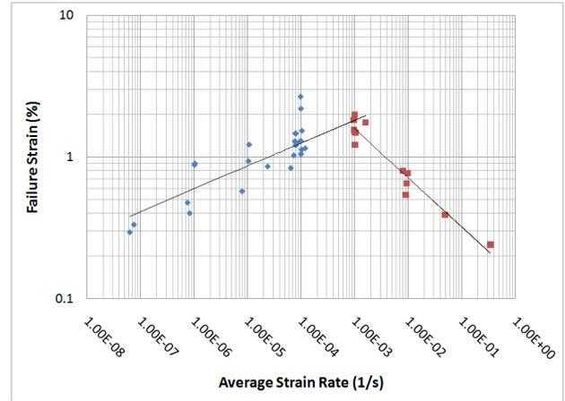
Figure 6. Variation of Failure Strain with Strain Rate in Tension for Fairbanks Silt
