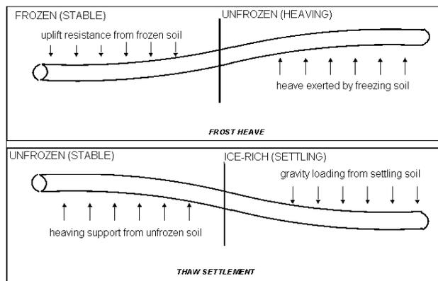
Figure 1. Conceptual Illustration of Freezing Thawing Effects on Pipelines in Discontinuous Permafrost (Nixon, 1994)
