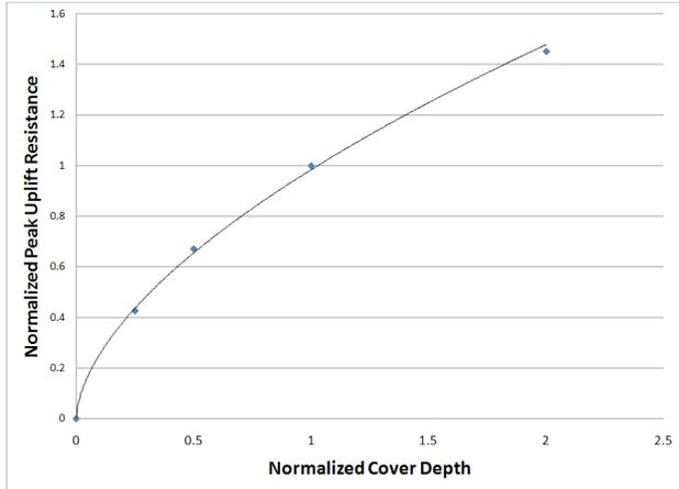
Figure 9. Normalized Peak Uplift Resistance Versus Normalized Cover Depth
