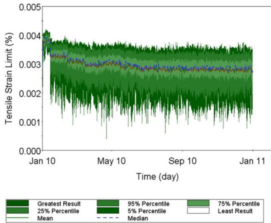
Figure 13. Variation of Tensile Strain Limit with Time
