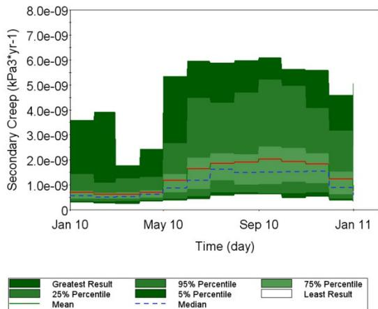
Figure 14. Variation of Creep Parameter B with Time.
