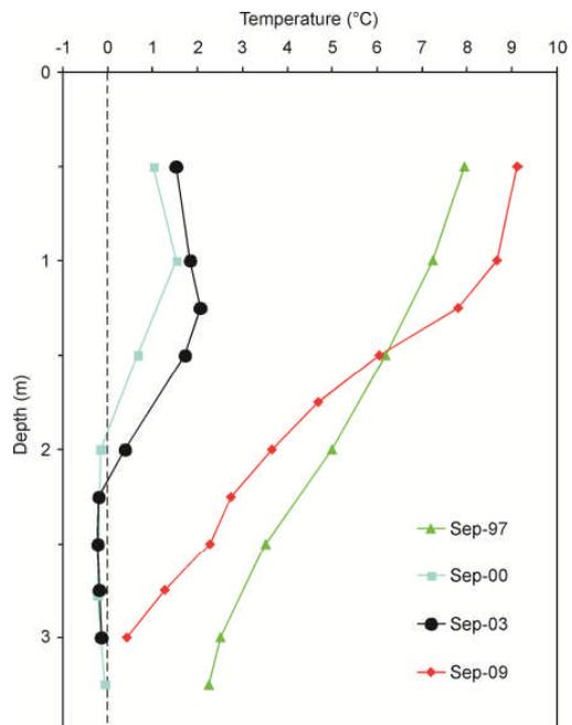
Figure 9. Ground temperatures beneath the berm at KP5. Temperatures for 1997 are prior to berm placement.
