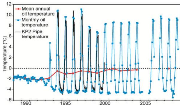
Figure 2. Monthly and mean annual oil temperatures exiting the Norman Wells pump station and mean daily external pipe wall temperatures at KP2.
