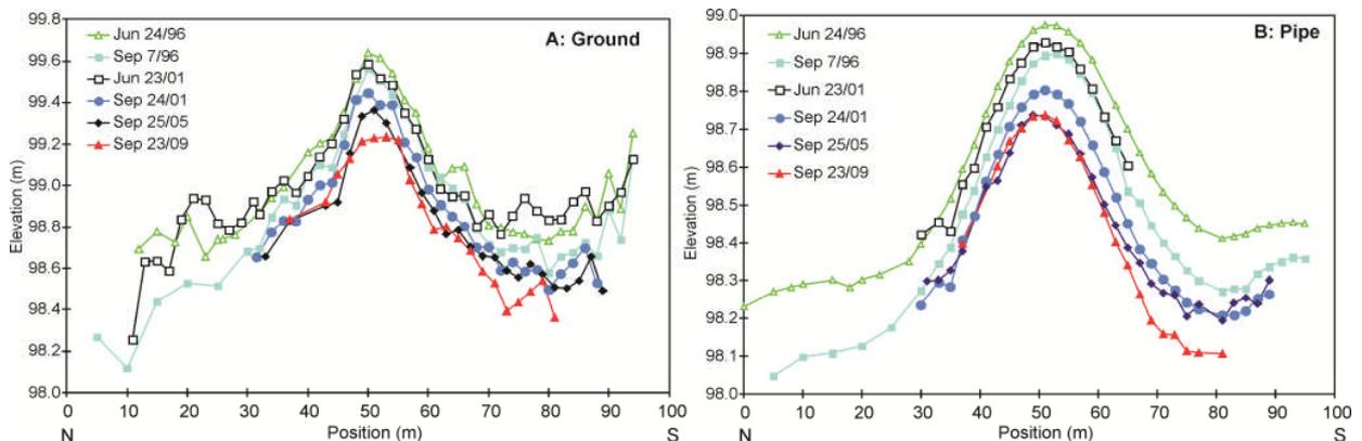
Figure 5. Ground surface (A) and Pipe (B) elevation (relative to local datum) at KP2 for selected dates during the monitoring period. N and S refer to pipeline north and south respectively. Note different vertical scales for A and B.
