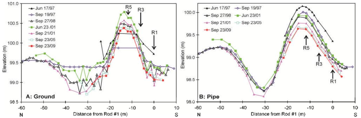
Figure 7. Ground (A) and pipe (B) elevation (relative to local datum) at KP5 for selected dates. N and S refer to pipeline north and south respectively. Rod positions shown in Figure 8 are indicated by R1, R2, R3. Note, vertical scales for A and B are different.
