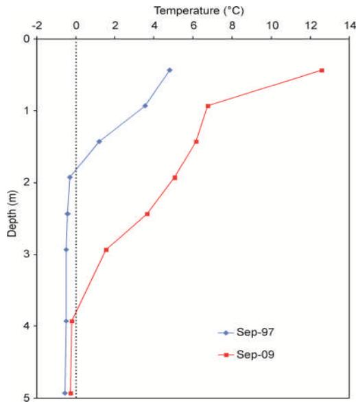
Figure 4. Ground temperatures at KP2 at pipeline south end of site (80 m position).
