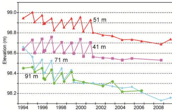
Figure 6. Pipe elevation (relative to local datum) over time at selected locations at KP2. Note spring and fall surveys prior to 2001; fall only thereafter.
