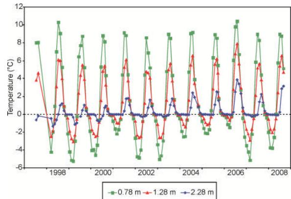
Figure 3. Mean monthly ground temperatures for depths to 2.3 m near KP12, a cleared firebreak adjacent to the town of Norman Wells.
