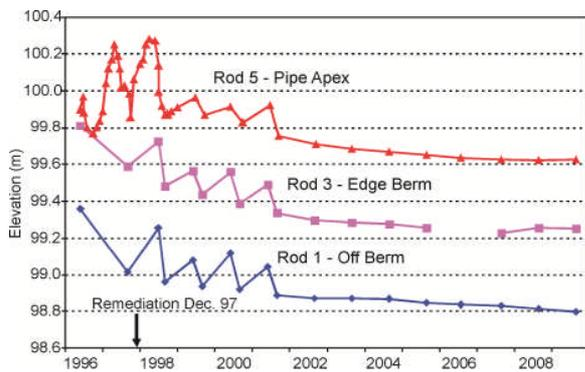
Figure 8. Pipe elevation (relative to local datum) over time at selected positions at KP5. See Figure 7 for rod location. Higher frequency measurements were made by Enbridge at Rod 5 at the beginning of the monitoring period. Note, only fall measurements after 2001.
