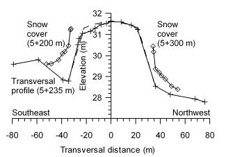
Figure 8. Elevation of the embankment surface on July 2004 and snow surface on April 2005 on the Southeast and Northwest shoulders and toes of the airfield embankment at Tasiujaq Airport, Northern Quebec, Canada. The dash line is the transversal profile as built (MTQ 1990). Note the vertical exaggeration 1:40.
