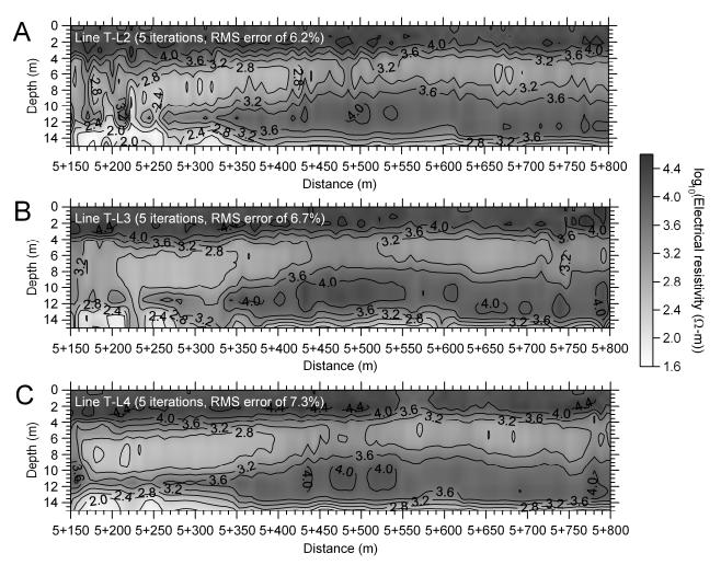
Figure 10. Models of electrical resistivity along the survey lines T-L2 (A), T-L3 (B), and T-L4 (C) over the Southeast side, center line and Northwest side of the airfield embankment respectively at Tasiujaq Airport, Northern Quebec, Canada. See Figure 3 for the location of survey lines T-L2, T-L3, and T-L4. Note the vertical exaggeration (1:10).
