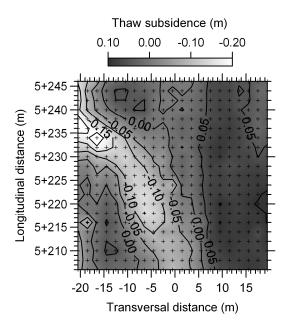
Figure 4. Spatial distribution of thaw subsidence affecting the airfield embankment near the distance 5+230 m, Southeast side, on July 2004 at Tasiujaq Airport, Northern Quebec, Canada. The + symbols identify the location of elevation measurements.
