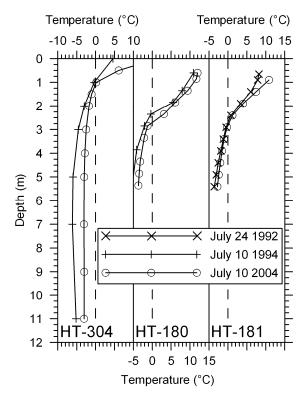
Figure 6. Temperature profiles in the field (HT-304) and in the airfield embankment and subgrade (HT-180 and HT-181) at Tasiujaq Airport, Northern Quebec, Canada. See Figure 3 for the location of thermistor cables HT-304,
