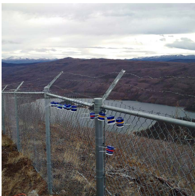
Figure 3. Mercury passive air samplers at Little Fox Lake
