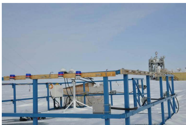
Figure 2. Mercury passive air samplers at Alert
