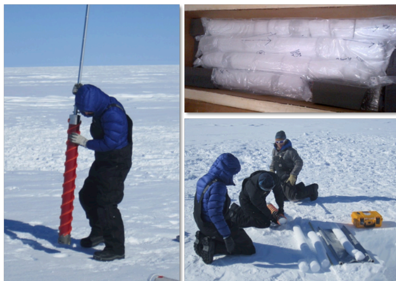
Figure 2. Ice core drilling and sampling.
