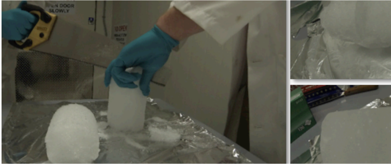
Figure 3. Ice core sectioning and images of ice layers.
