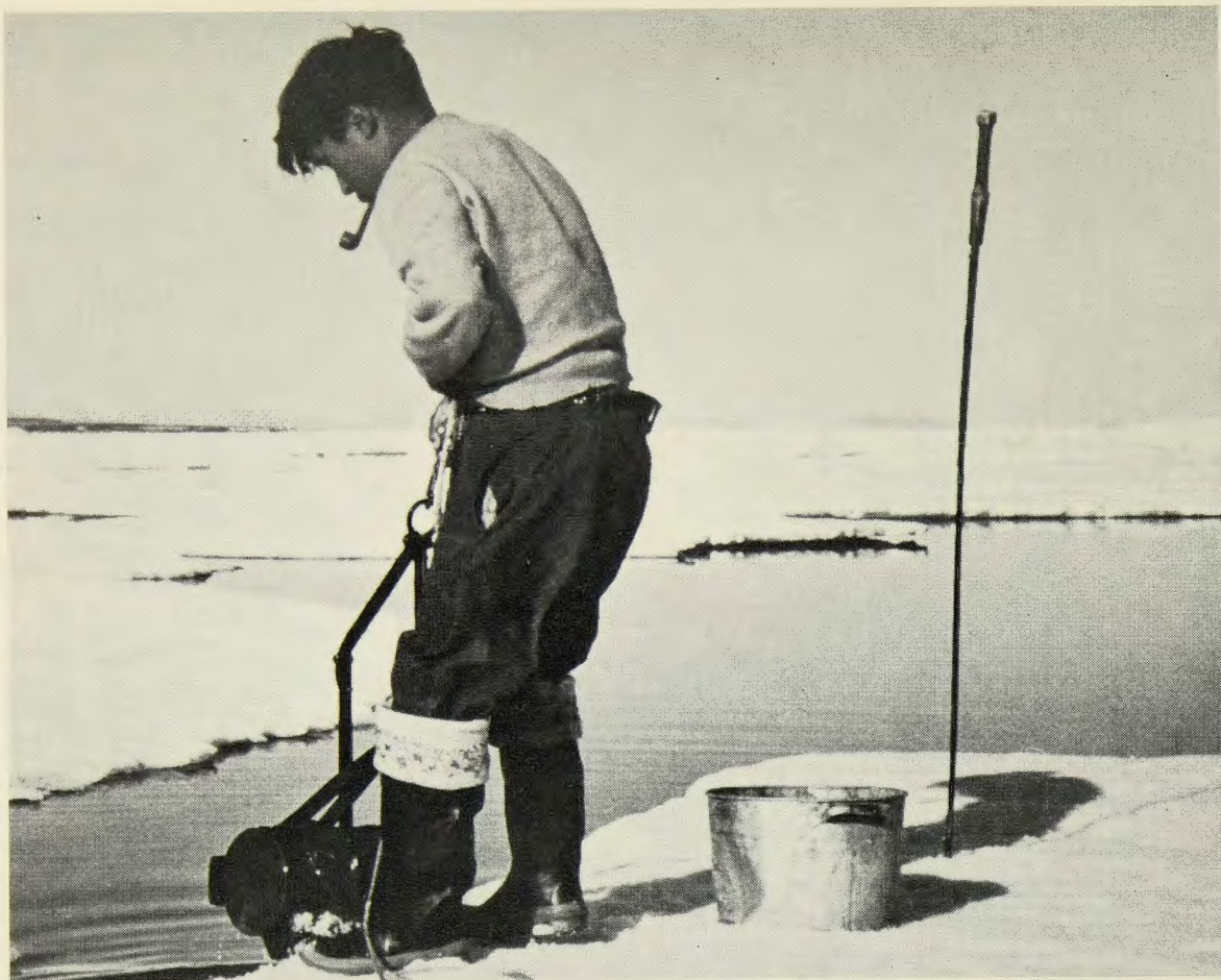
Pl. 1. Foerst grab with a haul of benthos being pulled on to sea ice in Eclipse Sound.
