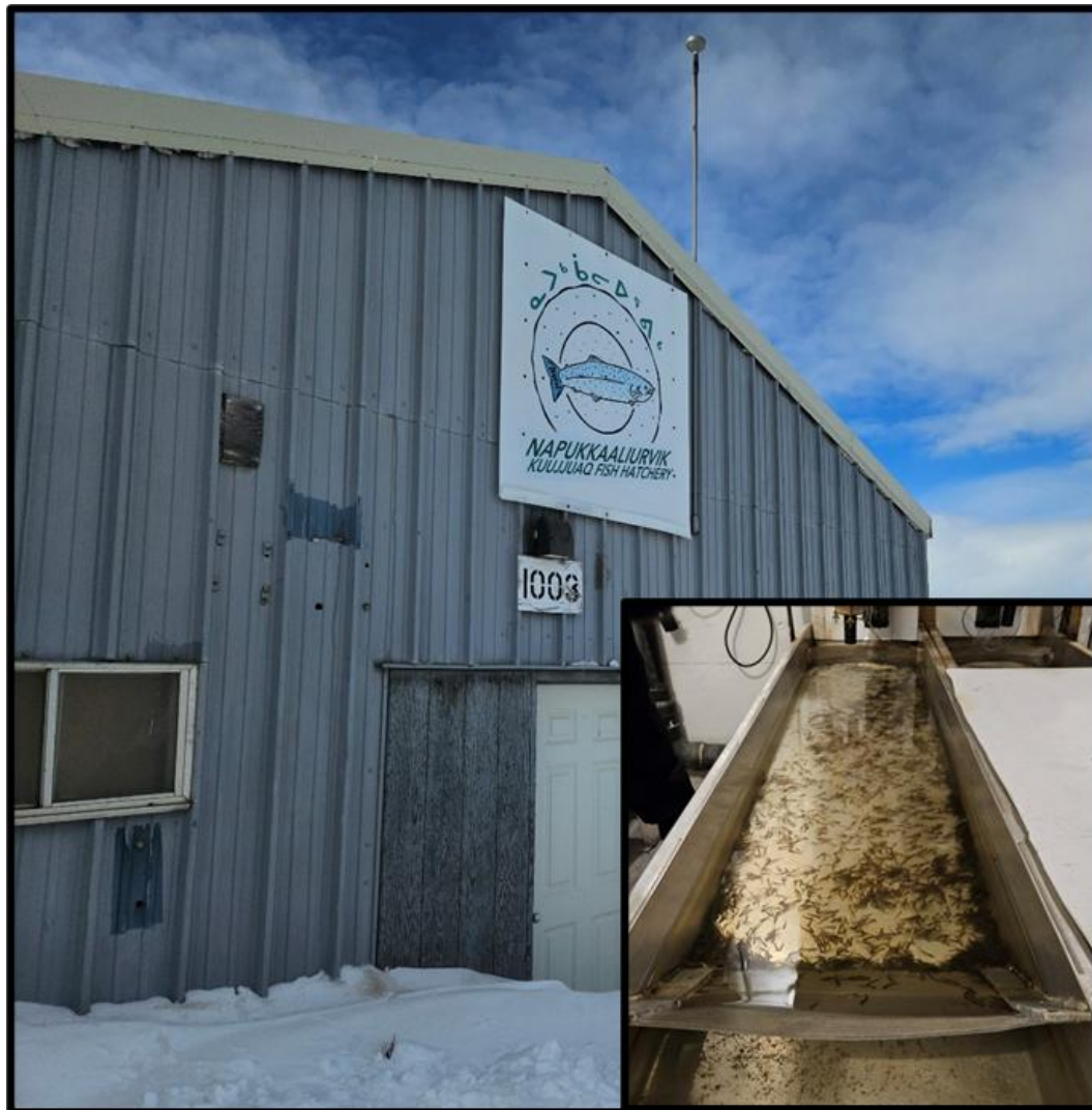
Figure 7: The Napukkaaliurvik Kuujjuaq Fish Hatchery in Kuujjuaq, Nunavik (19 th March 2025). Insert: tray containing char alevins, fed and oxygenated on a timer to maintain regular and predictable rates of growth.
