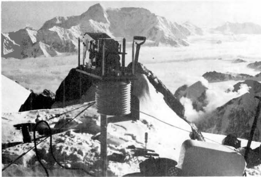
Fig. 10. One-year temperature and pressure recorder installed by CRREL at 5600 m. on Mt. Logan. The view is south across the Seward Glacier basin to Mt. St. Elias, 5489 m. Photo by Joseph LaBelle.
