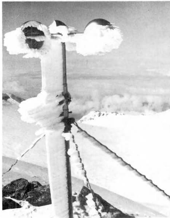
Fig. 11. Rime accumulation on totalizing anemometer, 5600 m., Mt. Logan. Rime and frost growth seriously impair observation at unmanned sites in this environment. Photo by Joseph LaBelle.
