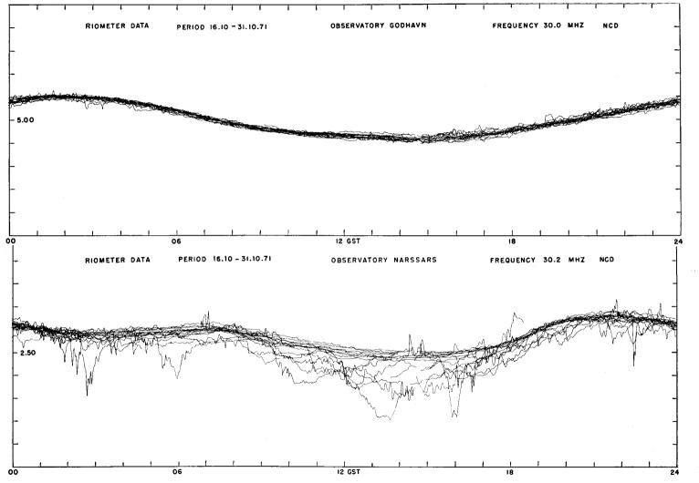
FIG. 3. Massplots of riometer recordings from a transauroral station (Godhavn), and an auroral station (Narssarssuaq) showing the strong variations in auroral absorption.
