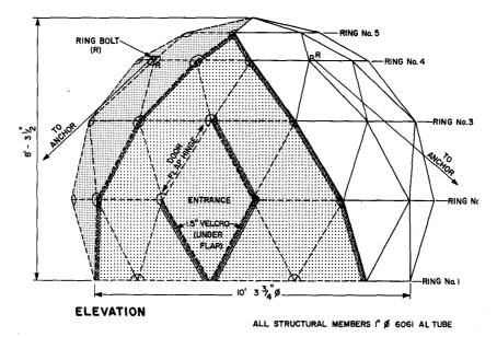
FIG. 2. Plan and elevation of the dome showing cut-away view of main canopy. Outer neoprene nylon canopy is not shown. For details see text. Frame detail courtesy of Triodetic\* Building Products Ltd., Ottawa.
