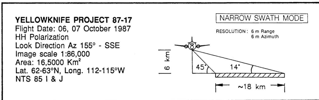
FIG. 1. Operating geometry of CCRS C-band radar in narrow swath mode.
