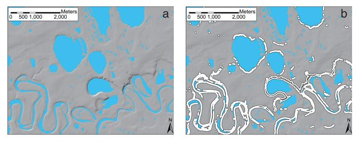
FIG. 4. Examples of IfSAR DTM data in the National Petroleum Reserve – Alaska. (a) Hill shading is used to increase the visibility of terrain changes. Abrupt changes in landscape are indicated by extreme dark or extreme light shading. (b) Polar bear denning habitat, identified by white lines highlighted with a black border, occurred mostly along stream banks and lakeshores.
