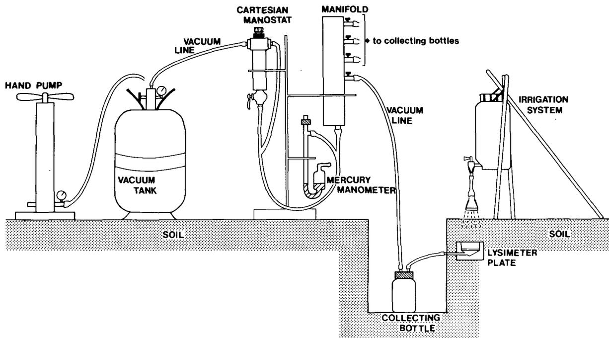
FIGURE 2. Tension lysimeter apparatus.
