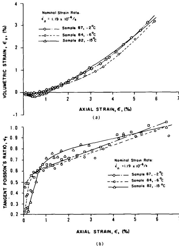
FIGURE 5. Temperature effect on constant strain-rate compression test results (after Bragg 1980). a Volumetric strain vs. axial strain. b Tangent Poisson's ratio vs. axial strain.
