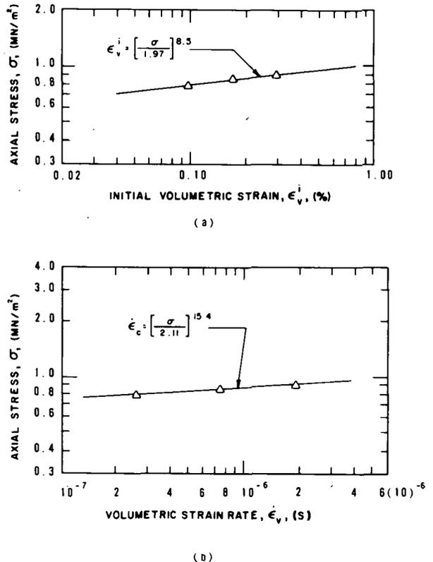
FIGURE 7. a Instantaneous volumetric strain vs. axial stress. b Volumetric strain rate vs. axial stress.
