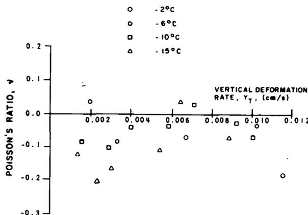
FIGURE 10. Poisson's ratio versus applied vertical deformation rates for the indirect tensile test (after Bragg 1980).
