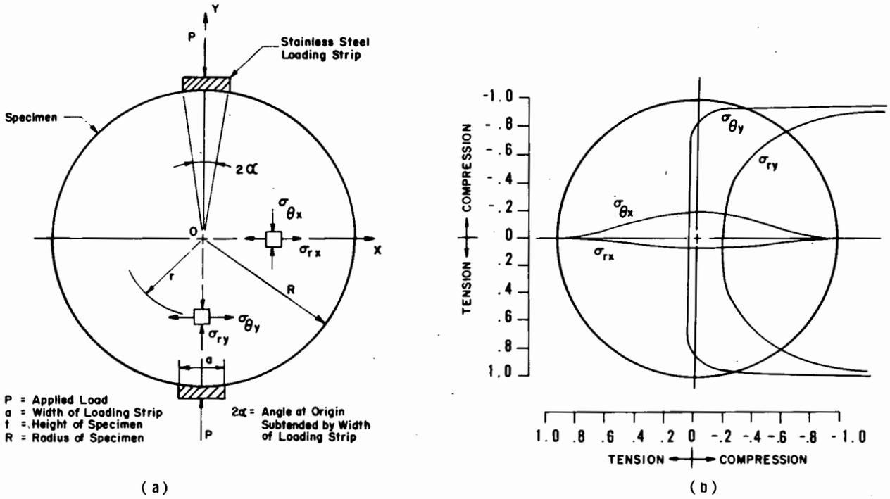
FIGURE 1. Indirect tensile test. a Loading conditions. b Stress distribution (after Hondros 1959).
