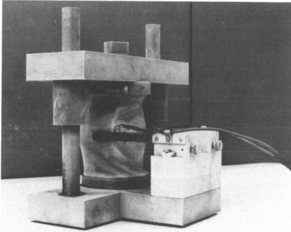
FIGURE 3. Loading apparatus and horizontal deformation transducer for the indirect tensile test.
