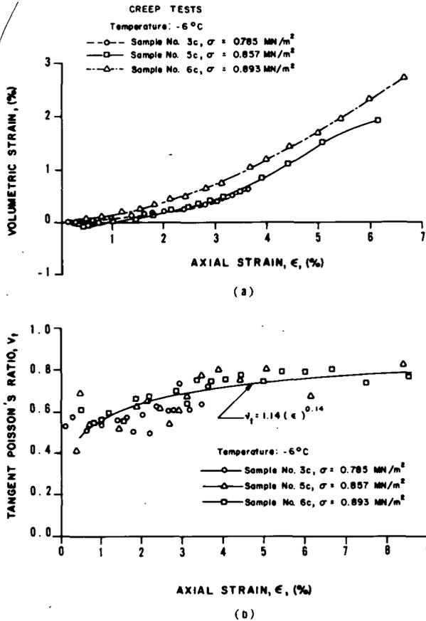
FIGURE 8. Constant stress (creep) test results (after Bragg 1980). a Volumetric strain vs. axial strain. b Tangent Poisson's ratio vs. axial strain.
