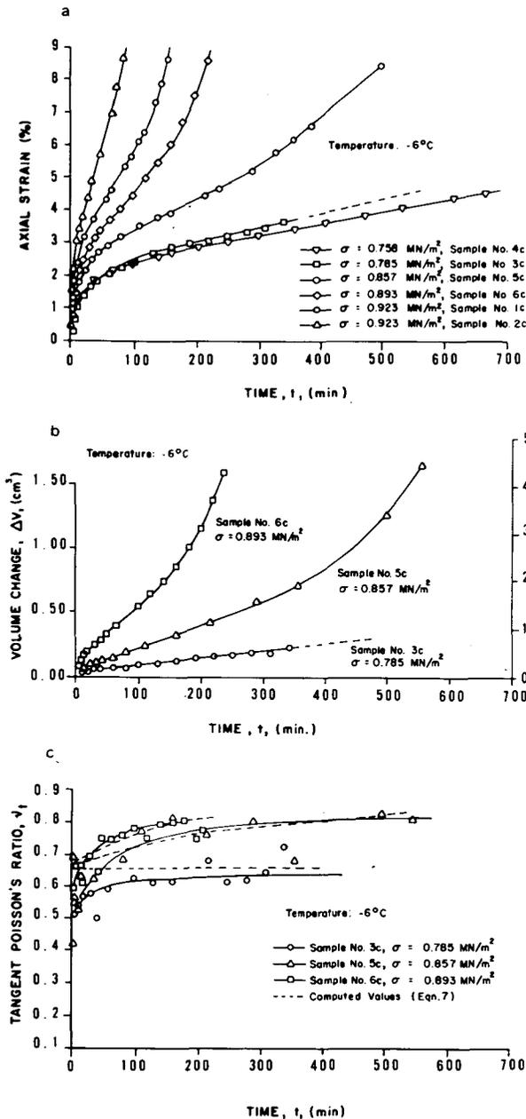
FIGURE 6. Constant stress compression (creep) test results (after Bragg 1980). a Axial stress vs. time. b Volume change vs. time. c Tangent Poisson's ratio vs. time.
