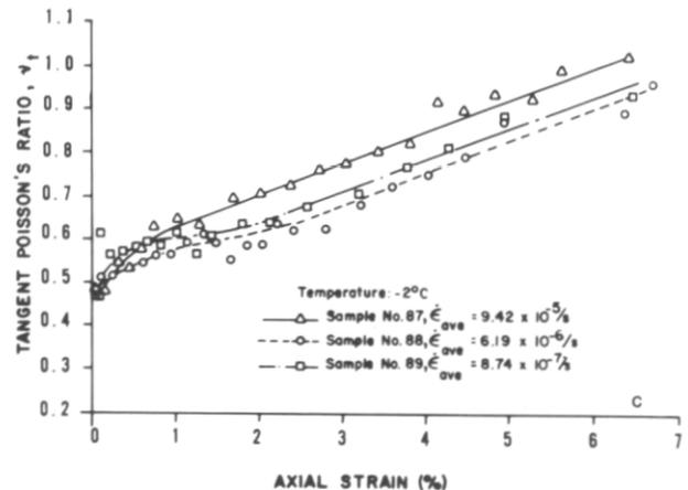
FIGURE 4. Constant strain-rate compression test results at  $-2^{\circ}\text{C}$  (after Bragg 1980). **a** Stress vs. axial strain. **b** Volumetric strain vs. axial strain. **c** Tangent Poisson's ratio vs. axial strain.
