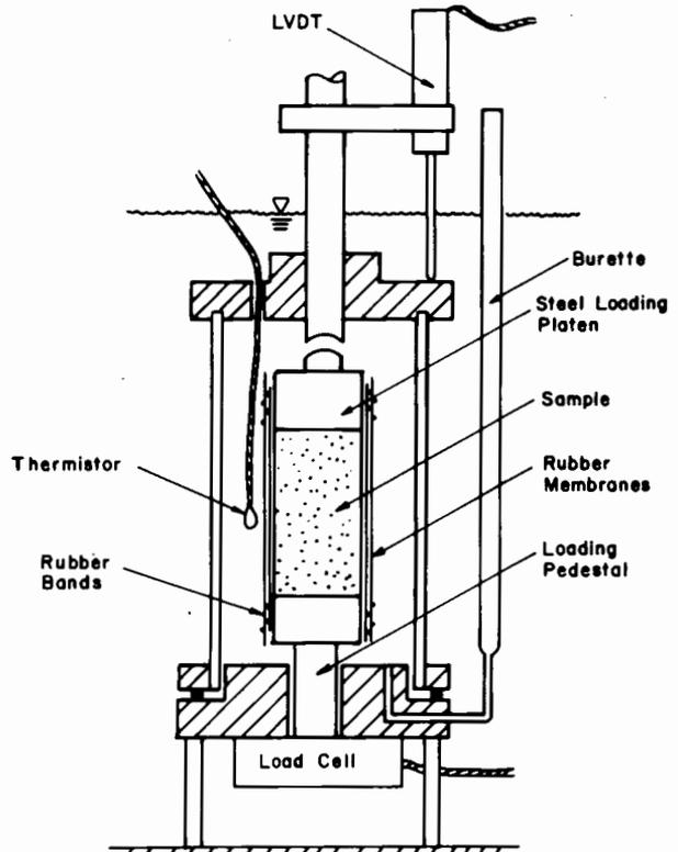
FIGURE 2. Schematic diagram of the triaxial cell.
