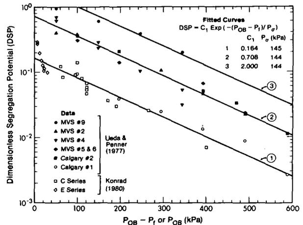
FIGURE 3. Experimental data fitted to an exponential law dependence of dimensionless segregation potential ( $DSP$ ) on overburden pressure.
