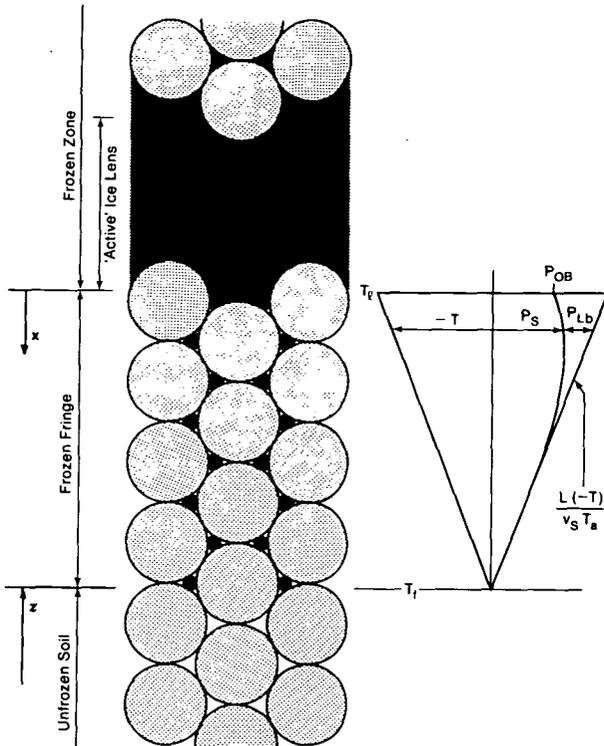
FIGURE 1. Schematic representation of a frozen fringe in a soil consisting of spherical particles. Temperature and pressure dependences through the fringe are shown on the right.
