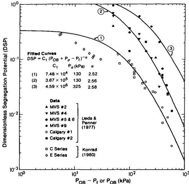
FIGURE 2. Experimental data fitted to a power law dependence of dimensionless segregation potential ( $DSP$ ) on overburden pressure.
