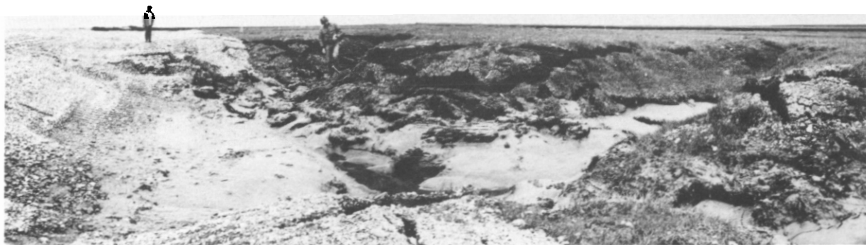
FIGURE 1. Massive sinkhole adjacent to the buried pipeline. This is a polygonal ground area where the workpad and pipeline intersect ice wedge.
