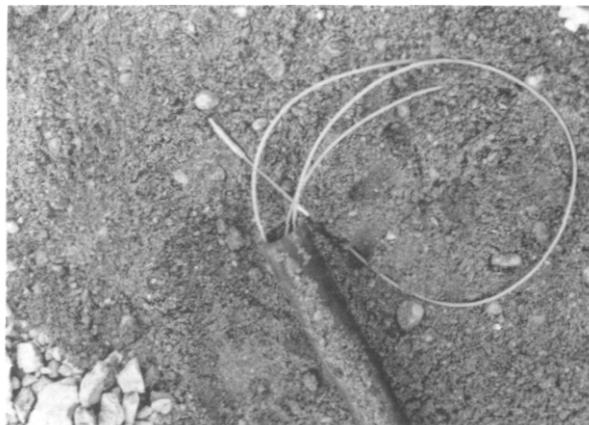
FIGURE 11. Close-up of thermistor.
