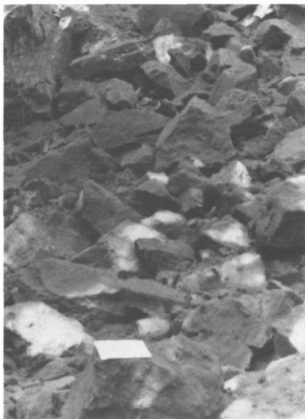
FIGURE 2. A typical example of poor fragmentation in frozen material.
