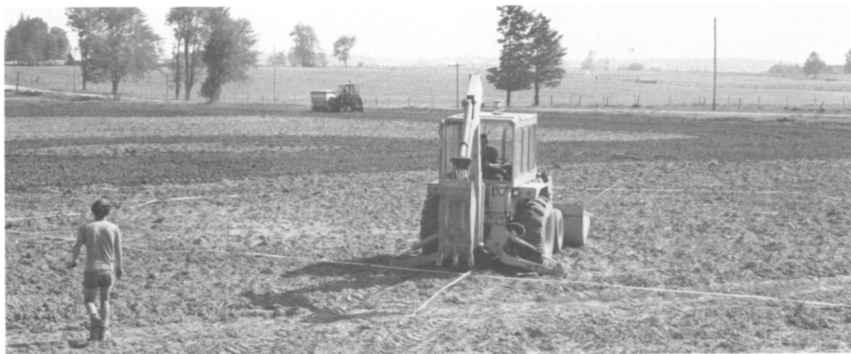
FIGURE 6. The Muir polygons being trenched. Photographed only six hours after Figure 5, the polygon outlines have disappeared due to strong evaporation from the soil surface. Surveying tape placed perpendicular to the polygon boundary, aligns the trench to cut across the polygon. The machine is about to cut Wedge #4.
