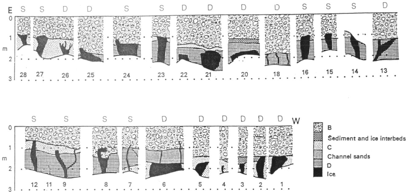
Figure 2. Stratigraphic setting of ice bodies mapped at the reservoir in 1986. Horizontal and vertical scale is the same. Classification of shallow (S), and deep (D) ice bodies refers to groups described in the text. B, C, and D refer to stratigraphic units described in the text.
