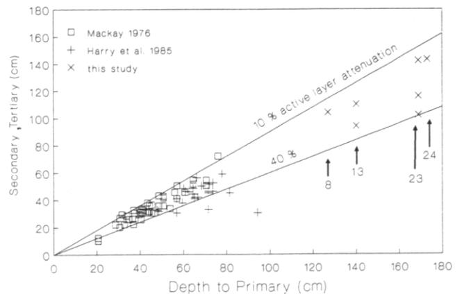
Figure 4. Comparison of the depth to primary, secondary and tertiary ice wedge surfaces in the eastern and western Arctic. Numbers refer to specific ice wedges shown in Figure 2.
