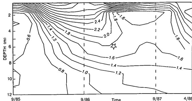
Figure 4. Mean annual geotherms for cable T3 (on-ROW) at site 85-11, km 597. Dashed lines are 1 year apart. Time on x-axis represents mid point of year for a given mean annual temperature. Plot runs from Sept. 1985 to April 1988. Star denotes depth of penetration of 1986 "hump".
