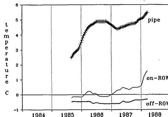
Figure 3. Running mean annual pipe and ground temperatures at nominal 1 m depth (see text). a) Site 84-3B, b) Site 85-7A, and c) Site 85-10B.
