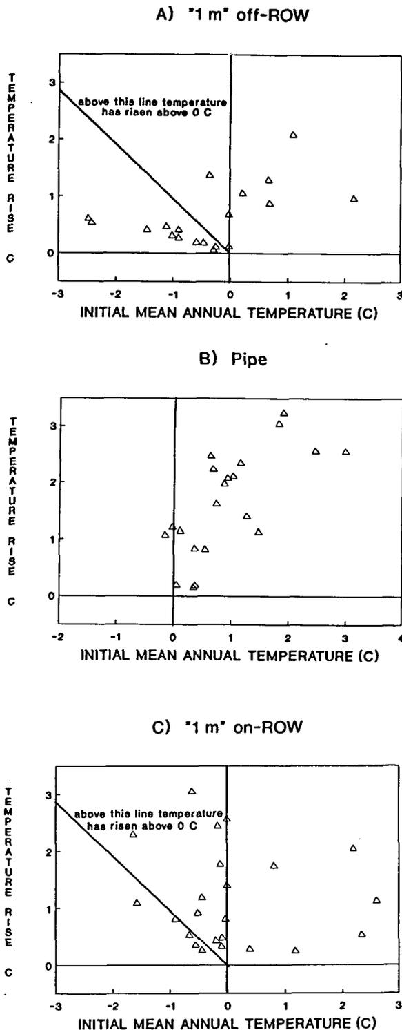
Figure 5. Thermal response (change in mean annual temperature over observation period for sites showing warming) as a function of initial mean annual temperature: a) "1 m" off-ROW, b) pipe, and c) "1 m" on ROW.
