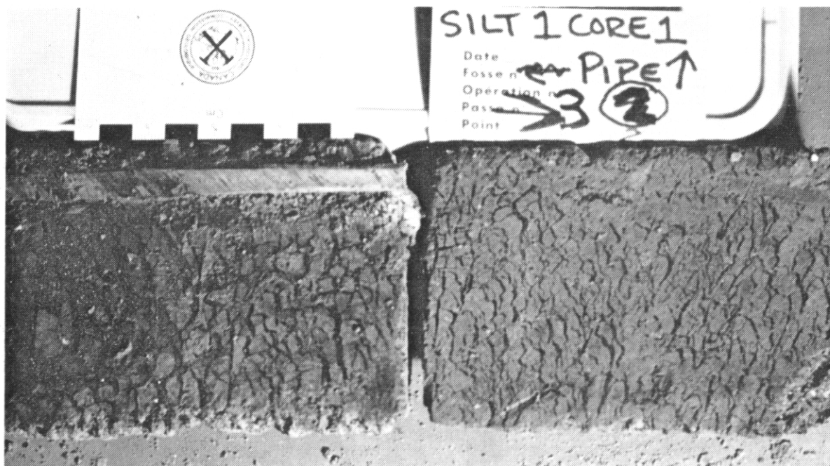
Figure 3. Ice blades next to the pipe at site 1, 50 to 80 cm below the surface. The pipe is on the left side of the photograph.
