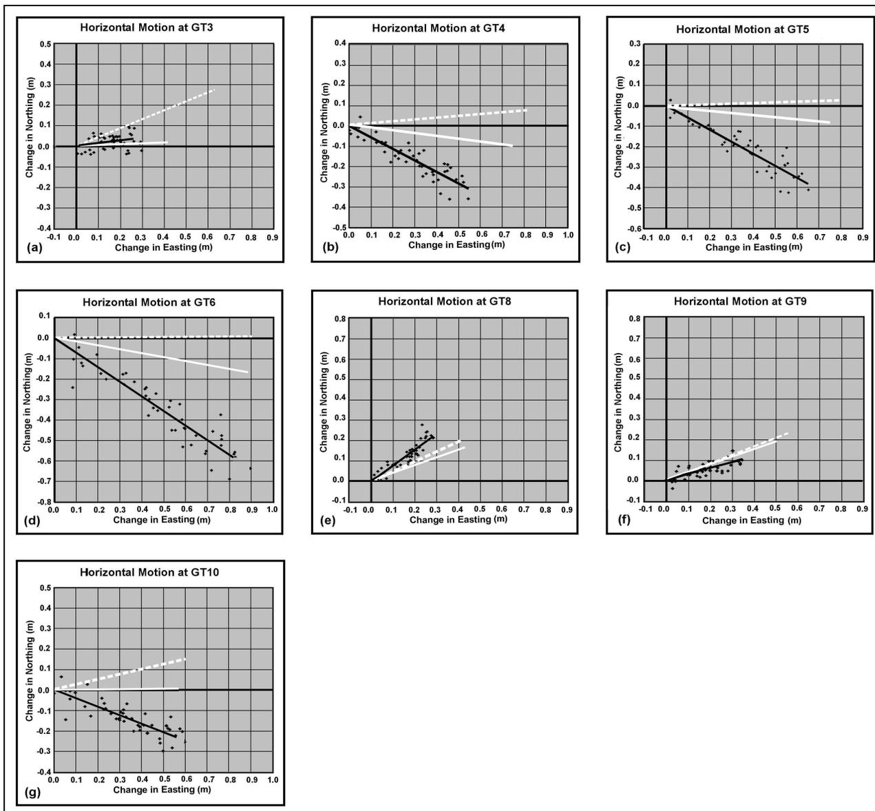
Figure 2: Measurement of horizontal displacement over 59 days. The black dots represent individual photogrammetric measurements, with the black line being fitted by regression. The continuous white line represents measurements derived by GPS, whereas the dashed white line represents average displacements derived from SAR interferometry.
