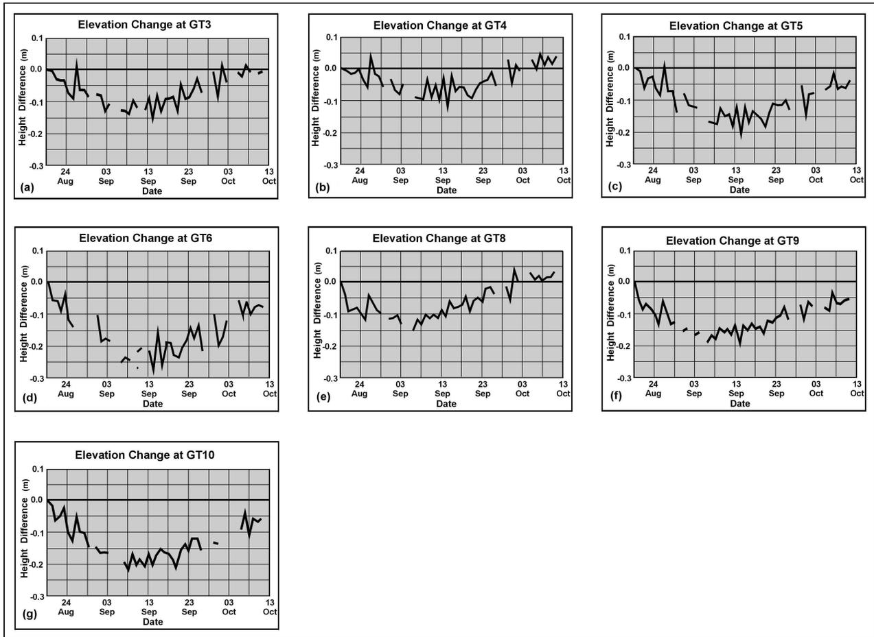
Figure 3: Vertical motion of the glacier surface over 59 days derived from photogrammetric measurements. The observations have been corrected to account for down-glacier motion.
