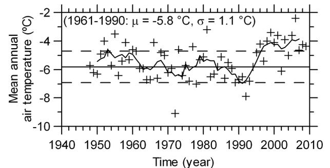
Figure 5. Mean annual air temperature at Kuujjuaq (meteorological record from Environment Canada, <http://climate.weatheroffice.gc.ca/index.html>). The full curve is a 5 year running average while the full and dashed horizontal lines are respectively the average and  $\pm$  standard deviation (values in parentheses) over the reference period 1961–1990.
