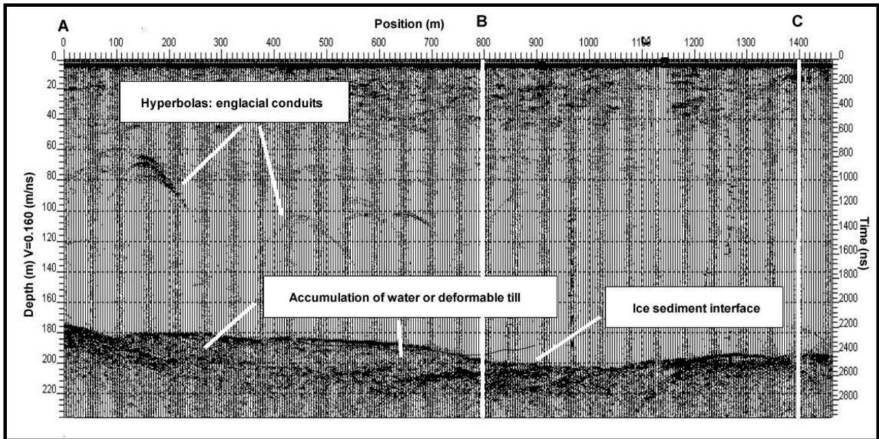
Figure 4: Annotated GPR trace showing the reflections at the glacier bed which were interpreted as being from a body of subglacial water or saturated till. The location of points A, B, and C can be seen on Figure 1b.
