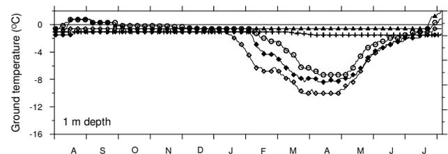
Figure 8 Top of permafrost temperatures for undisturbed tundra ( $\diamond$ ), sump caps with low snow (D43 ( $\circ$ ), B19 ( $\blacklozenge$ )), and high snow (C42 ( $+$ ), H54 ( $\blacktriangle$ )) in 2005/2006. Symbols are plotted at 6-day intervals for clarity (modified from Kokelj et al. 2010, Figure 5).
