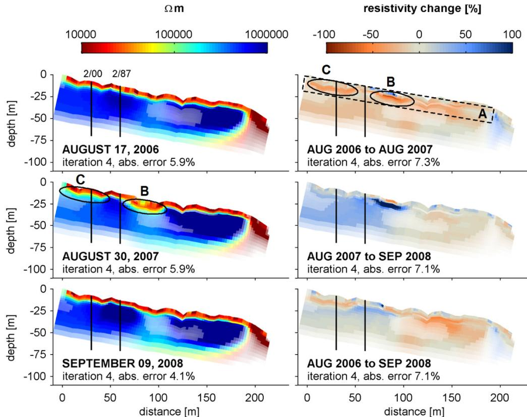
Figure 8. (left) ERT inversion models with intensity of colours scaled by the DOI index and (right) time-lapse tomograms scaled by  $DOI_{max} > 0.2$  for the Murtèl-Corvatsch rock glacier data sets (modified after Hilbich et al., 2009). The pale colours are associated with unreliable inversion results. Highlighted zones A, B and C are described in the text. The locations of boreholes 2/1987 and 2/2000 are shown as vertical lines on the right and left respectively.
