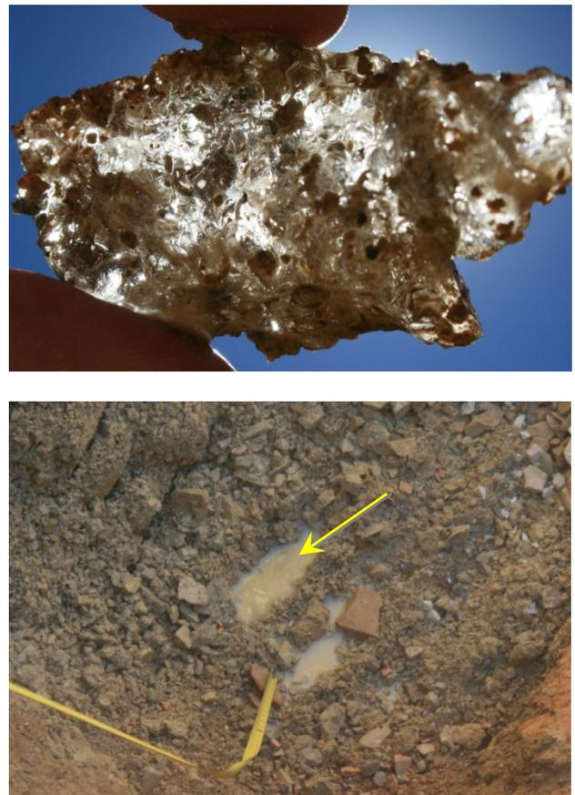
Figure 9. Sample from Test pit 2 (top). Also note the water flow on top of permafrost table (arrow).
