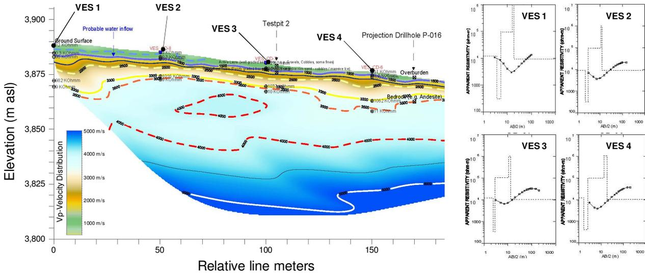
Figure 12. Surface refraction tomography and VES results. Survey carried out in the centre of rock glacier #2, perpendicular to the flow line. The figure only shows the east half of the survey. Drillhole P-016 is located 20 m from the survey line.
