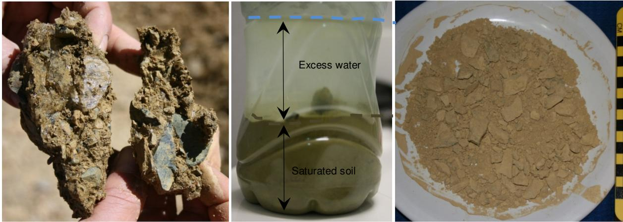
Figure 10. a) frozen, b) thawed and c) dry grab sample (~3m depth) from Test pit 2 at upper zone of Rock Glacier #2.
