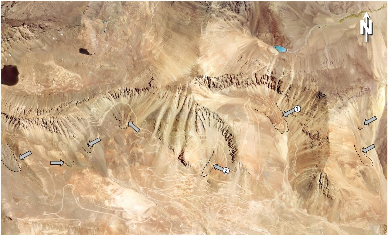
Figure 2. Aerial view of parts of the project area (section is approximately 4.7 km x 2.8 km). Various rock glaciers and protalus ramparts are indicated with arrows. Rock glaciers 1 and 2 are the focus of this study.
