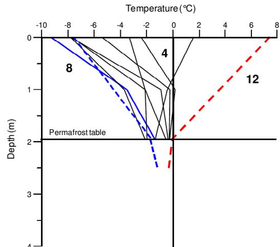
Figure 11. 2008 Rock glacier #1 ground temperature measurements. The dashed lines indicate an approximation of the estimated temperature range in the active layer.
