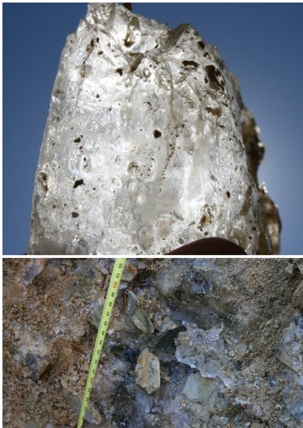
Figure 8. Samples from Test pit 1. Note the air bubbles and sandy - silty inclusions of the interstitial ice (top). The tape measure is in cm.
