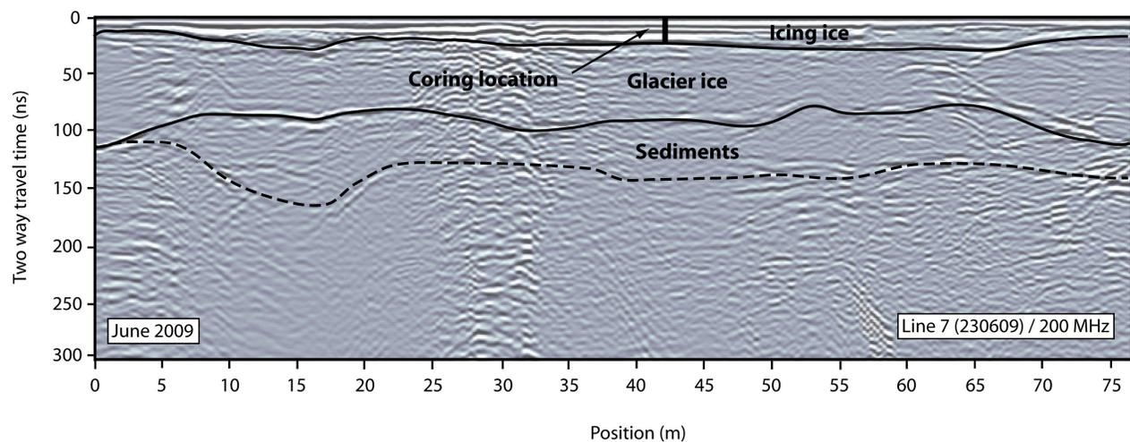
Figure 4. 200 MHz GPR line surveyed eastward following the centre line of the upper icing outwash plain. Survey was conducted in June of 2009.
