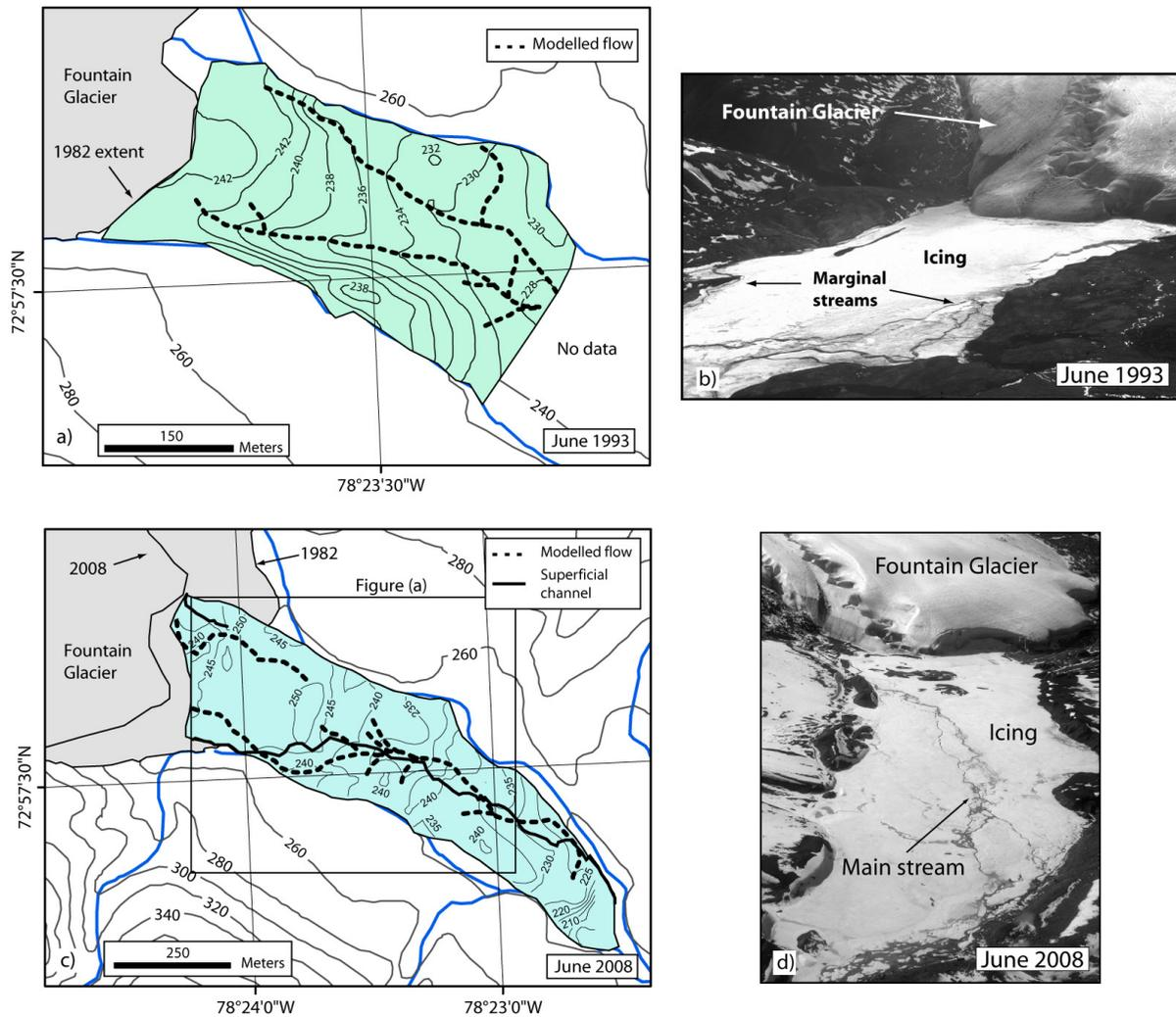
Figure 2. Meltwater streams within the proglacial icing have migrated from being marginal in 1993 to being central in 2008. a) and c) show the hydrological models generated from the surface and subicing DEMs, whereas b) and d) show oblique aerial photos of the modelled area. Field observations confirm the model results.
