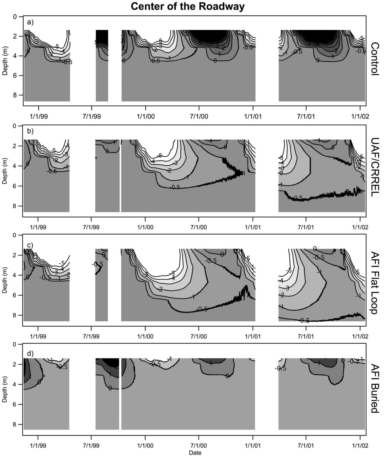
Figure 4. Center of the roadway ground temperature measurements from October 1998 to January 2002 at the a) control section, b) UAF/CRREL section, c) AFI flat loop section, and d) AFI buried section. The gray scale illustrates temperatures ( $^{\circ}\text{C}$ ) ranging from warm (black) to cold (white). Temperature contours shown are: -5, -4, -3, -2, -1, -0.5, 0, 1, 2, 3, 4, and 5  $^{\circ}\text{C}$ .
