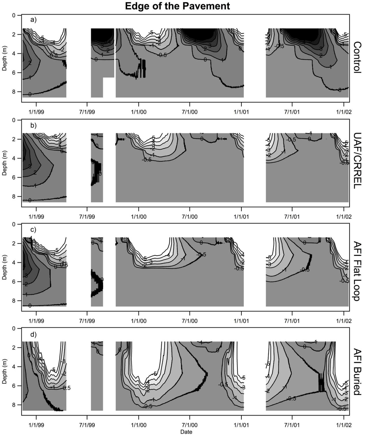
Figure 5. Edge of the pavement ground temperature measurements from October 1998 to January 2002 at the a) control section, b) UAF/CRREL section, c) AFI flat loop section, and d) AFI buried section. The gray scale illustrates temperatures (°C) ranging from warm (black) to cold (white). Temperature contours shown are: -5, -4, -3, -2, -1, -0.5, 0, 1, 2, 3, 4, and 5 °C.
