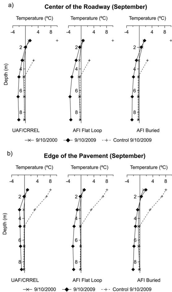
Figure 6. Whiplash curves on September 10 at a) the center of the roadway and at b) the edge of the pavement for years 2000 (solid cross) and 2009 (solid diamond). Dashed lines represent the temperature at the control section on September 10, 2009.
