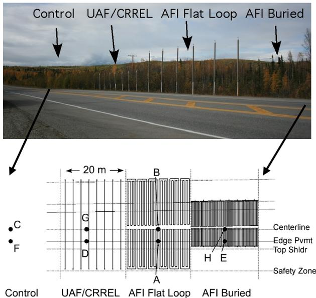
Figure 2. Layout of the installation including the control section, the UAF/CRREL section, the AFI Flat loop section, and the AFI Buried section. Four thermistor strings are located at the center of the roadway (C, G, B, H) and four strings at the edge of the pavement (F, D, A, and E).
