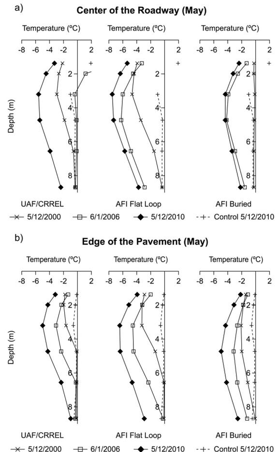
Figure 7. Whiplash curves on May 12 at a) the center of the roadway and at b) the edge of the pavement for years 2000 (solid cross), 2006 (open square) and 2009 (solid diamond). Dashed lines represent the temperature at the control section on May 12, 2010.
