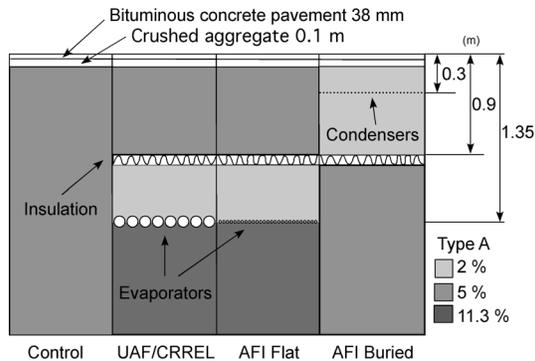
Figure 3. Cross section of the roadway installation. The gray scale illustrates water contents ranging from 2 % (light gray) 11.3 % (dark gray).
