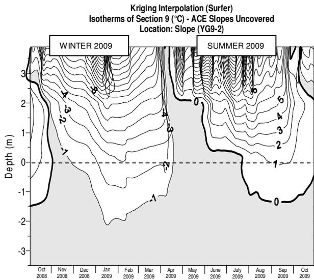
Figure 6 : Kriging interpolation thermal regime of the most efficient air convection embankment (section 9)
