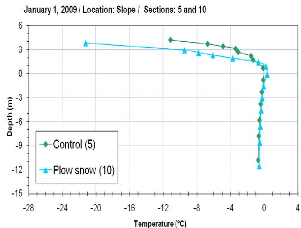
Figure 13: Thermal regimes of section 10 compared with the control section (January 1<sup>st</sup>, 2009)
