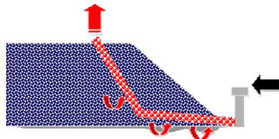
Figure 8: Conduction and convection air movements in the geocomposite
