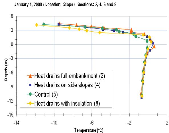
Figure 10: Thermal regimes of the heat drain sections compared with the control section (January 1<sup>st</sup>, 2009)
