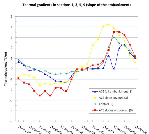
Figure 16: Thermal gradients ( $^{\circ}\text{C}/\text{m}$ ) calculated in the slopes of the air convection embankment sections
