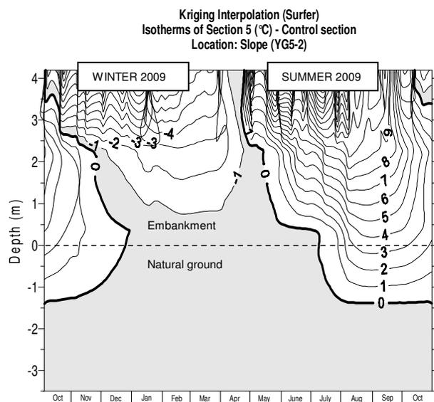
Figure 2: Kriging interpolation of the control section thermal regime
