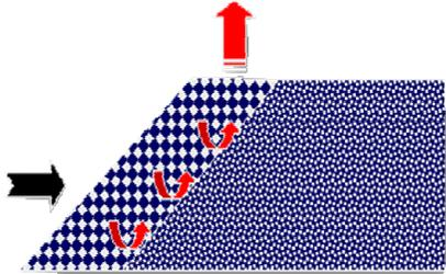
Figure 3: Air ascension in air convection embankment
