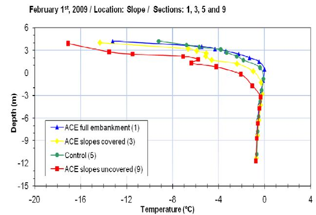
Figure 5: Thermal regimes in air convection embankment sections compared with the control section (February 1<sup>st</sup>, 2009)
