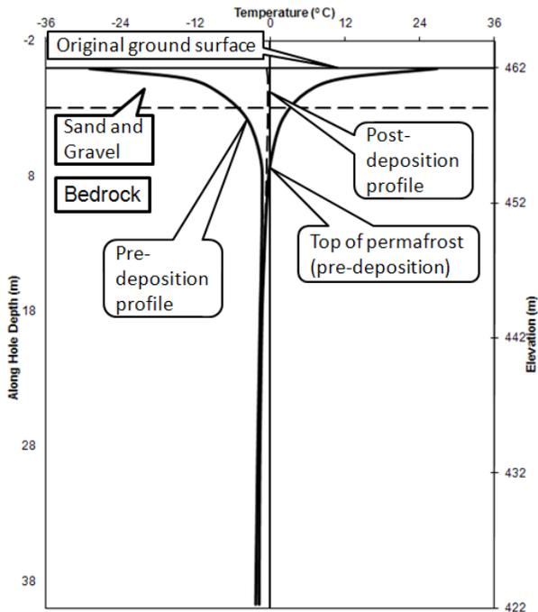
Figure 8. TH06-05: Pre- and post-deposition ground temperature profiles.
