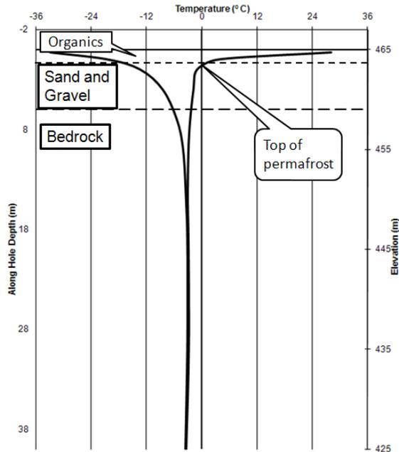
Figure 6. TH06-08: Pre-deposition ground temperature profile.
