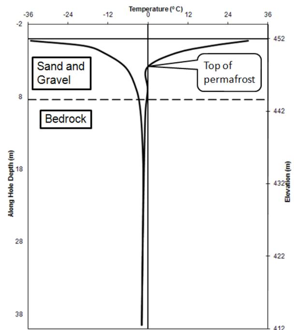
Figure 5. TH06-03: Ground temperature profile.
