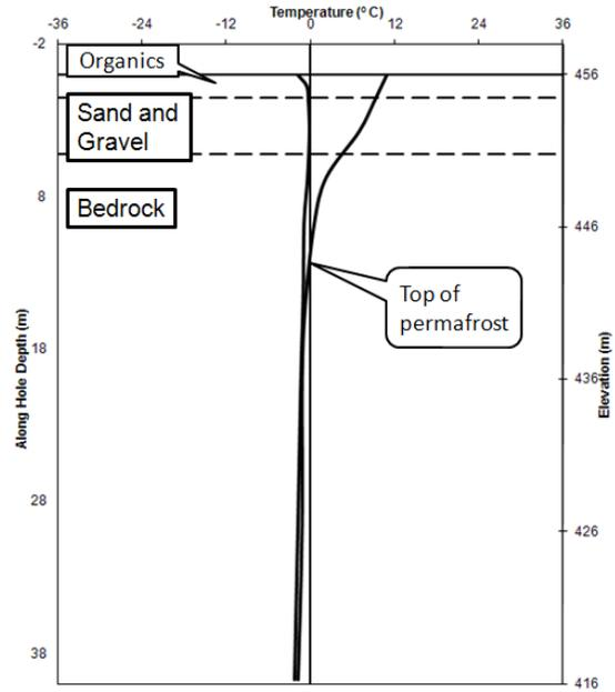
Figure 7. TH08-04 Ground temperature profile.
