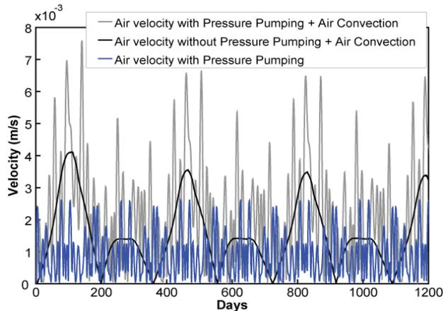
Figure 6. Air velocity at central line of 4 depths with varieties of boundary conditions
