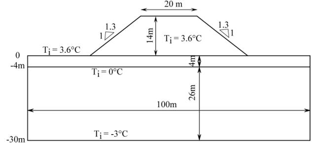
Figure 1. Schematic drawing of geometry and initial thermal conditions of the modeling waste rock pile
