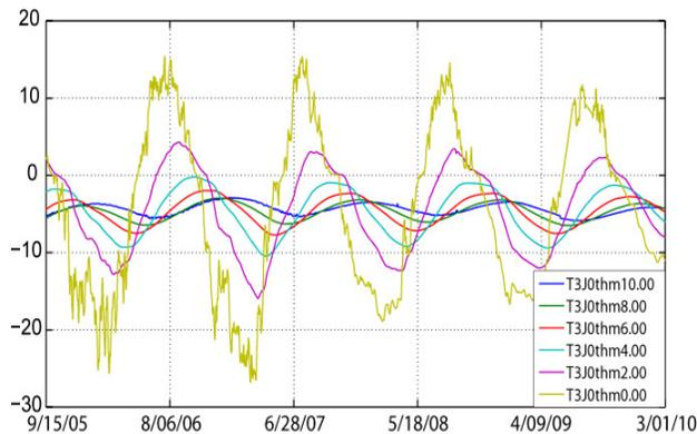
Figure 7. Bedrock temperature at different depths at Diavik mine
