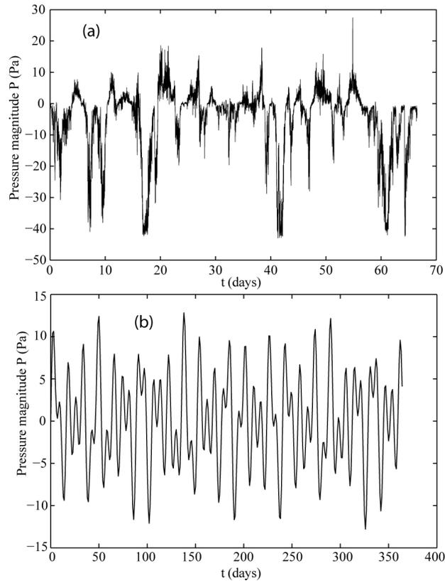
Figure 2. Measured pressure at a location of the surface of the pile (a) and simulated pressure (b) which is a combination of three sine functions
