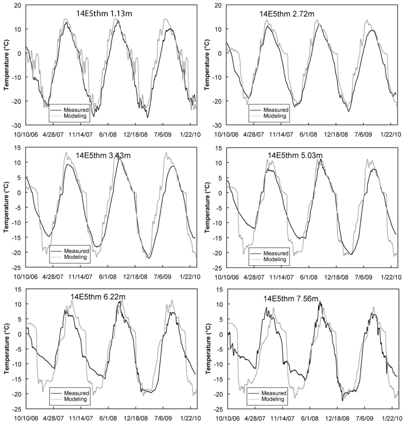
Figure 9. Measured and numerical modeling results of a waste rock pile's internal temperatures are up to 7.56m depth. The symbol 14E5thm 1.13m indicates a thermistor at type I pile, face 4, East of central line, 5 offset of central line and at 1.13m depth from the top surface, details of Diavik test pile project mentioned by Smith et al. (2009)
