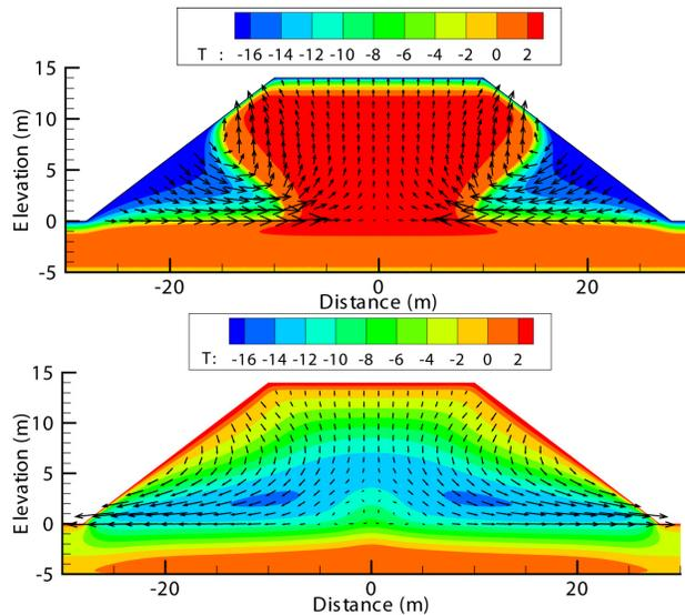
Figure 4. Contour plots showing air convection in winter (a) and conduction in summer (b)
