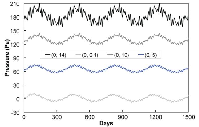
Figure 8. Pressure fluctuations at different points inside the waste rock pile
