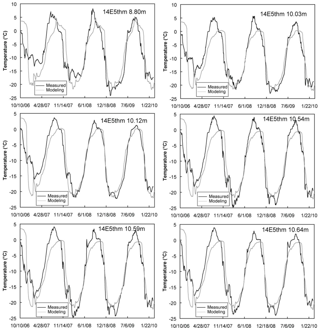
Figure 10. Measured and numerical modeling results of a waste rock pile's internal temperatures are from 8.80 to 10.64m depth
