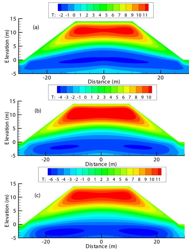
Figure 5. Contour plots of temperature after year 1 (a) year 2 (b) and year 3 (c)
